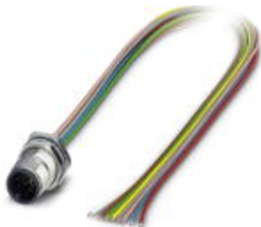
Sensor/actuator flush-type connector, 8-pos., M12 SPEEDCON, rear/screw mounting with M12 thread, with 0.5 m TPE litz wire, 8 x 0.25 mm 2
