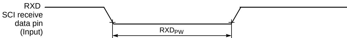
Figure 10-15 RXD Pulse Width
