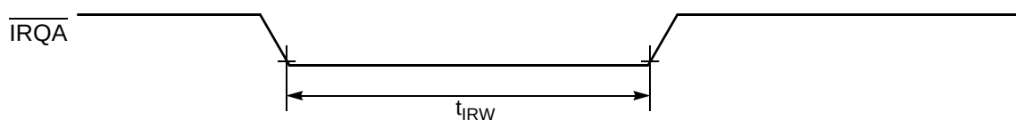
Figure 10-6 External Interrupt Timing (Negative Edge-Sensitive)
