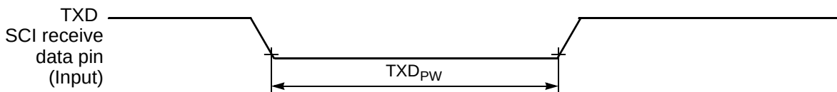
Figure 10-16 TXD Pulse Width
