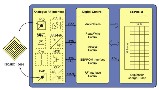
The label requires no internal power supply. Its contactless interface generates the power supply and the system clock via the resonant circuitry by inductive coupling to the interrogator. The interface also demodulates data that are transmitted from the interrogator to the I•CODE Label, and modulates the electromagnetic field for data transmission from the I•CODE Label to the interrogator.
