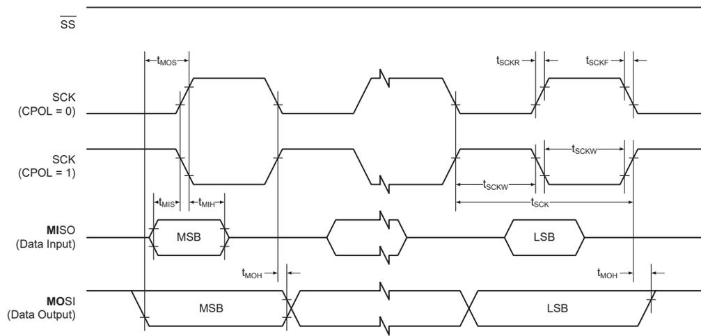
**Figure 37-5. SPI - Timing Requirements in Slave Mode**
