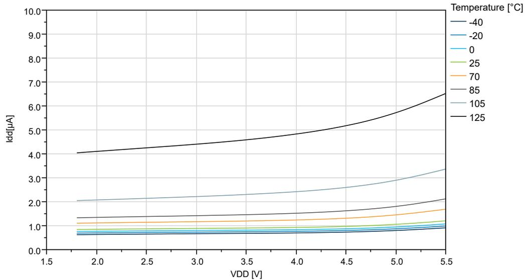
**Figure 38-13. ATtiny1614 Standby Mode Supply Current vs.  $V_{DD}$  (RTC Running with Internal OSCULP32K)**
