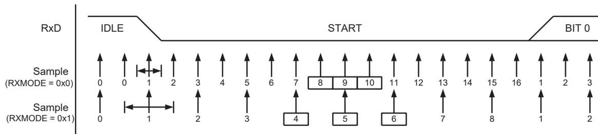
When the clock recovery logic detects a high-to-low (i.e., idle-to-start) transition on the RxD line, the Start bit detection sequence is initiated. Sample 1 denotes the first zero-sample, as shown in the figure. The clock recovery logic then uses three subsequent samples (samples 8, 9, and 10 in Normal mode, samples 4, 5, and 6 in Double-Speed mode) to decide if a valid Start bit is received:
