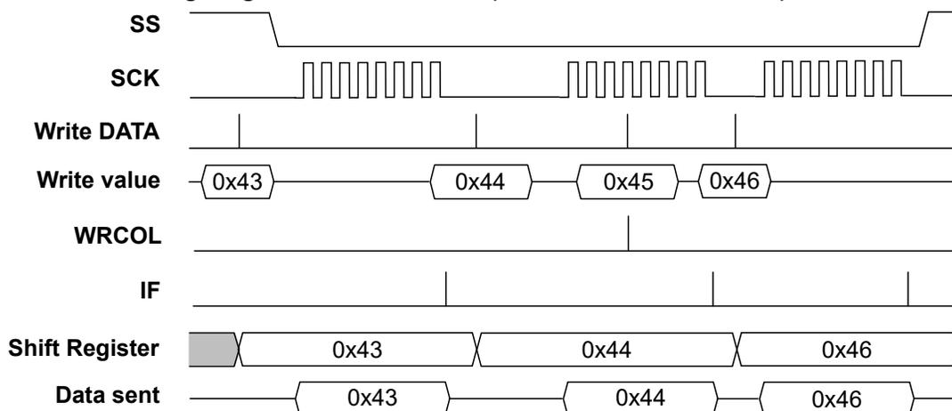
The figure above shows three transfers and one write to the DATA register while the SPI is busy with a transfer. This write will be ignored and the Write Collision Flag (WRCOL in SPIn.INTFLAGS) is set.
