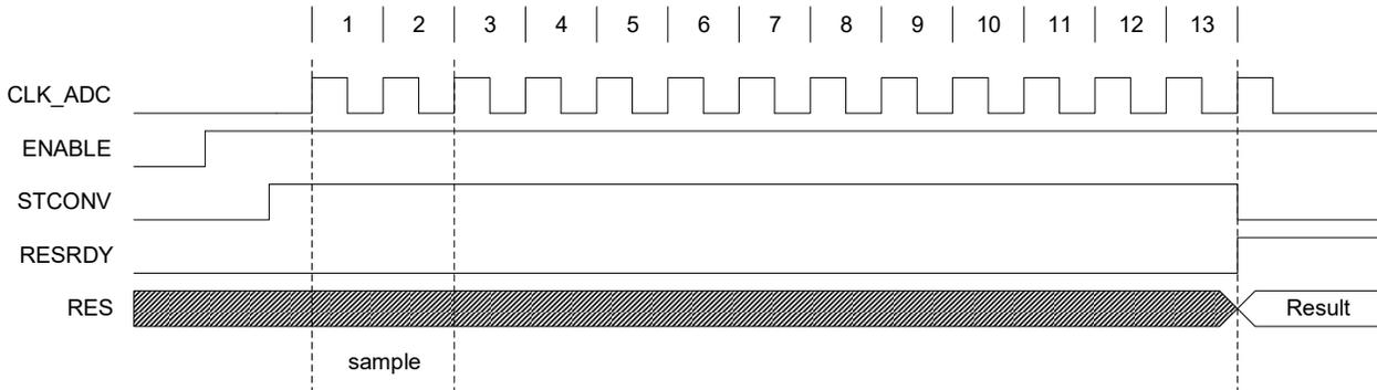
Both sampling time and sampling length can be adjusted using the Sample Delay bit field in Control D (ADC.CTRLD) and sampling the Sample Length bit field in the Sample Control register (ADC.SAMPCTRL). Both of these control the ADC sampling time in a number of CLK\_ADC cycles. This allows sampling high-impedance sources without relaxing conversion speed. See the register description for further information. Total sampling time is given by:
