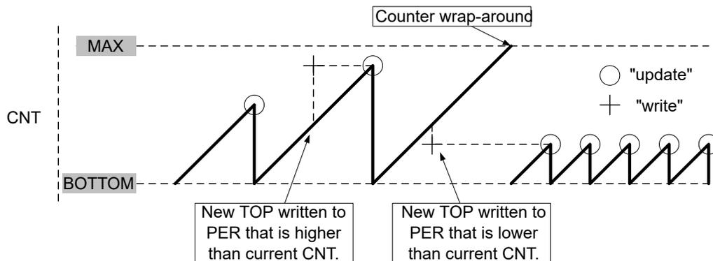
A counter wrap-around can occur in any mode of operation when up-counting without buffering. This is due to the fact that the TCA<sub>n</sub>.CNT and TCA<sub>n</sub>.PER registers are continuously compared: if a new TOP value is written to TCA<sub>n</sub>.PER that is lower than the current TCA<sub>n</sub>.CNT, the counter will wrap first, before a compare match happens.
