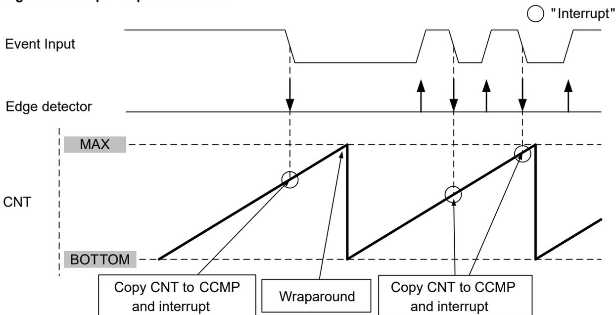
It is recommended to write '0' to the TCBn.CNT register when entering this mode from any other mode.
