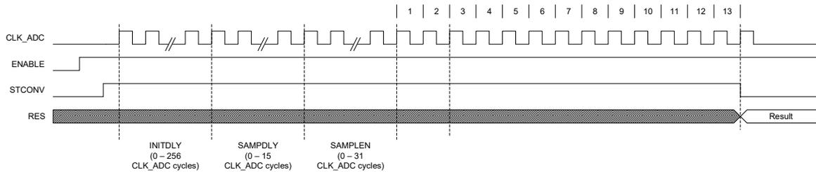
In Free-Running mode, a new conversion will be started immediately after the conversion completes, while the STCONV bit is '1'. The sampling rate  $R_S$  in free-running mode is calculated by:
