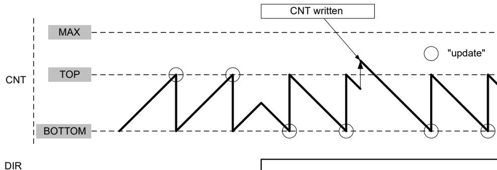
It is possible to change the counter value in the Counter register (TCA<sub>n</sub>.CNT) when the counter is running. The write access to TCA<sub>n</sub>.CNT has higher priority than count, clear, or reload, and will be immediate. The direction of the counter can also be changed during normal operation by writing to DIR in TCA<sub>n</sub>.CTRLA.
