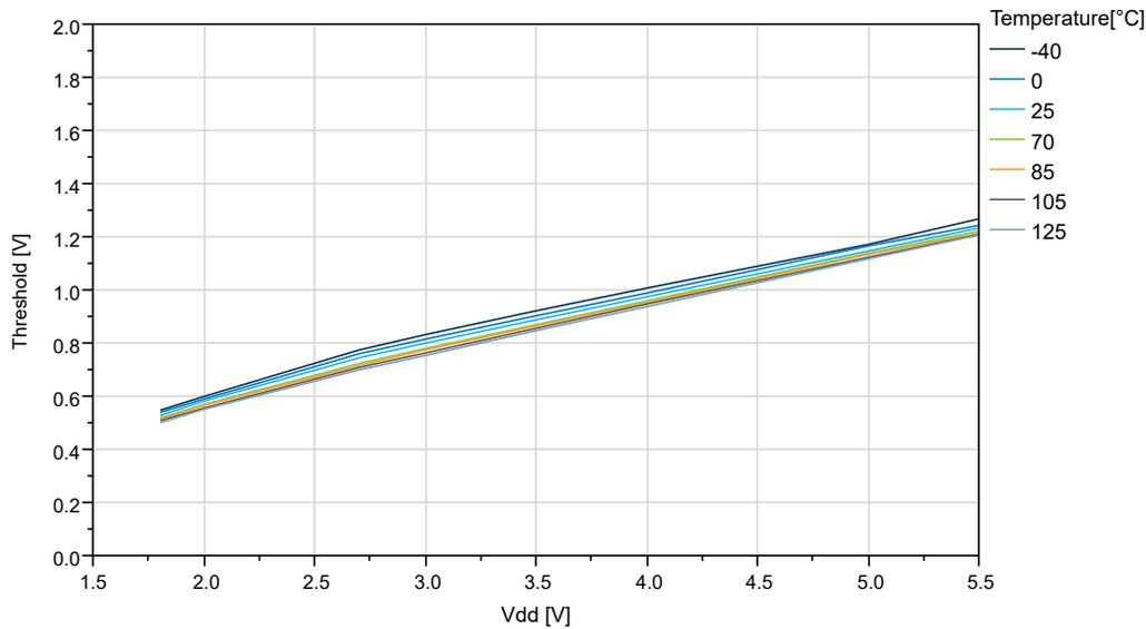
**Figure 38-17. I/O Pin Input Threshold Voltage vs.  $V_{DD}$  ( $T=25^{\circ}\text{C}$ )**
