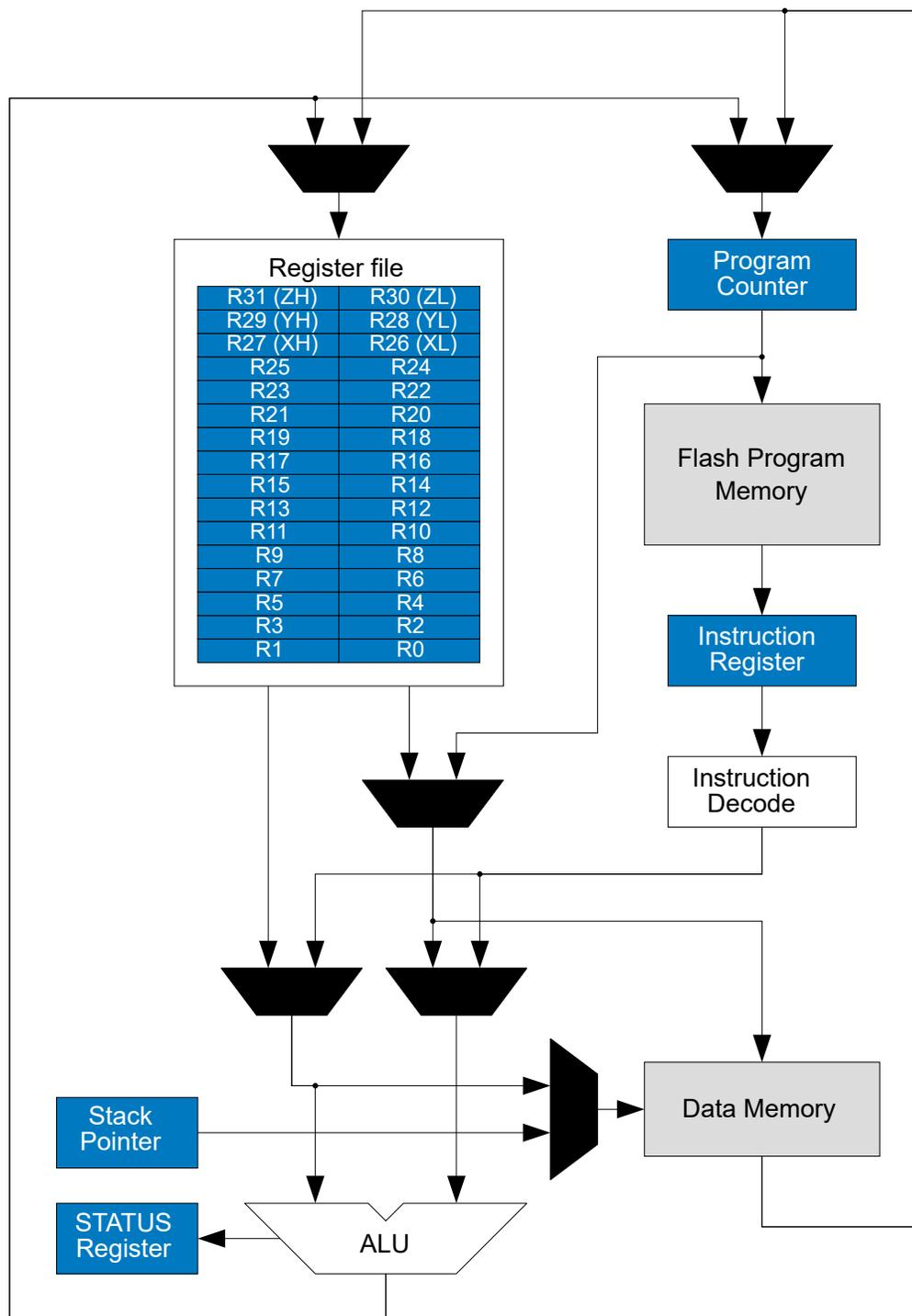
The Arithmetic Logic Unit (ALU) supports arithmetic and logic operations between registers or between a constant and a register. Also, single-register operations can be executed in the ALU. After an arithmetic operation, the STATUS register is updated to reflect information about the result of the operation.
