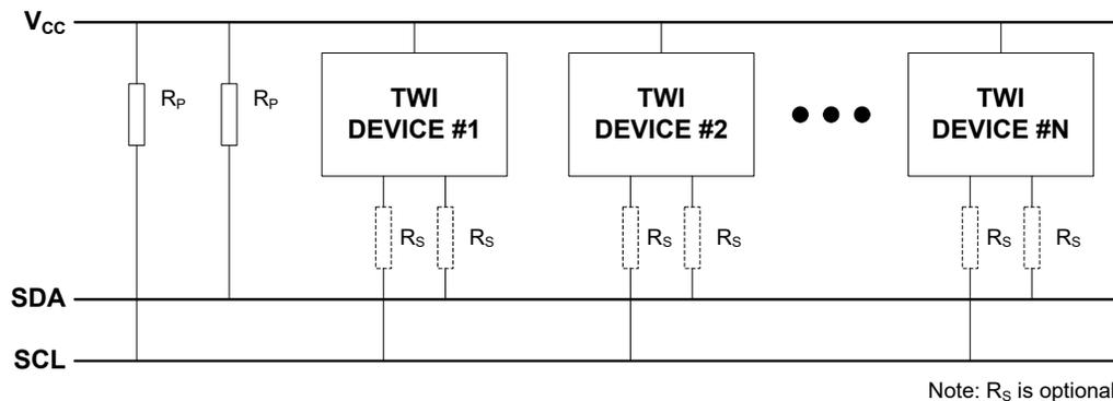
A unique address is assigned to all slave devices connected to the bus, and the master will use this to address a slave and initiate a data transaction.
