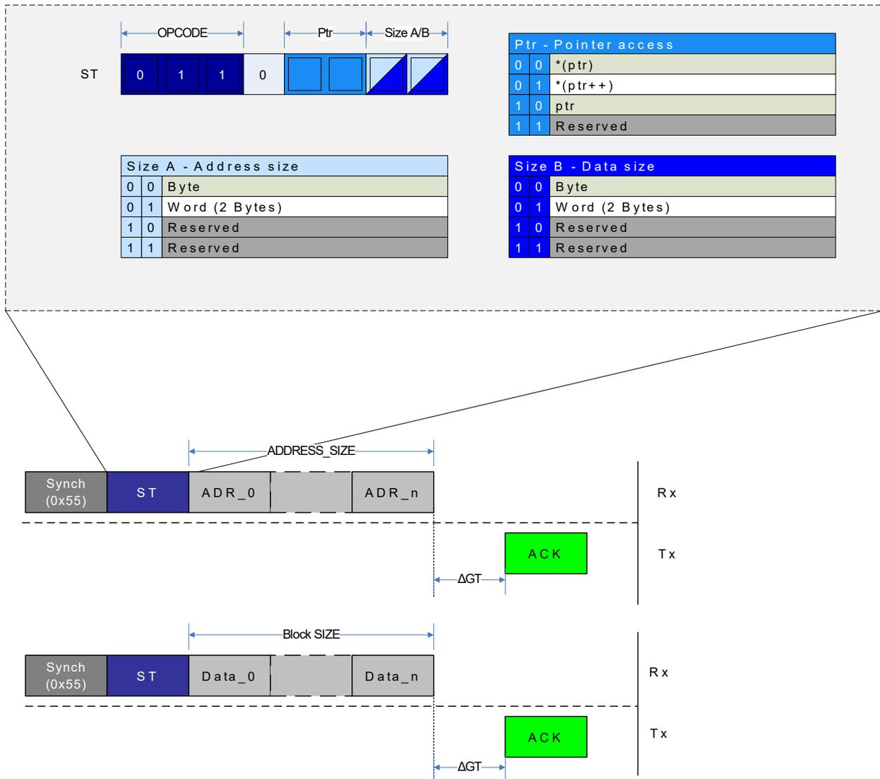
The figure above gives an example of `ST` to the UPDI Pointer register and store of regular data. In both cases, an Acknowledge (ACK) is returned by the UPDI if the store was successful and a SYNCH character is sent before each instruction. To write the UPDI Pointer register, the following procedure should be followed:
