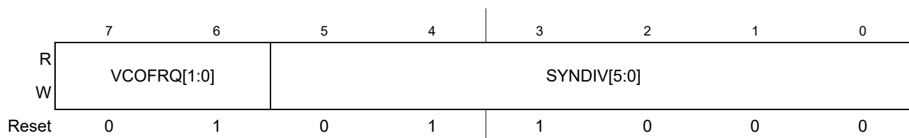
Figure 9-7. S12CPMU_UHV Synthesizer Register (CPMUSYNR)
