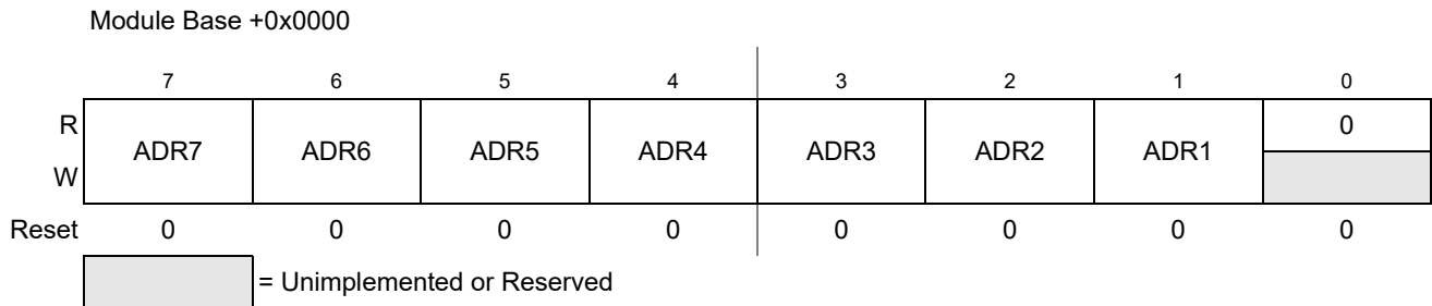
Figure 20-3. IIC Bus Address Register (IBAD)
