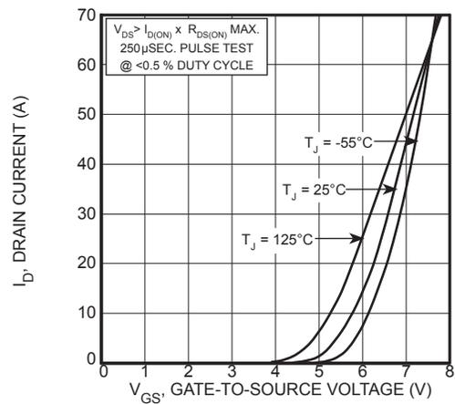
Figure 4, Transfer Characteristics
