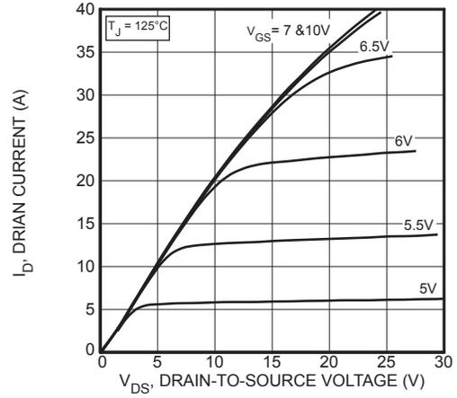
Figure 2, Output Characteristics
