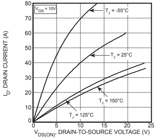
Figure 1, Output Characteristics
