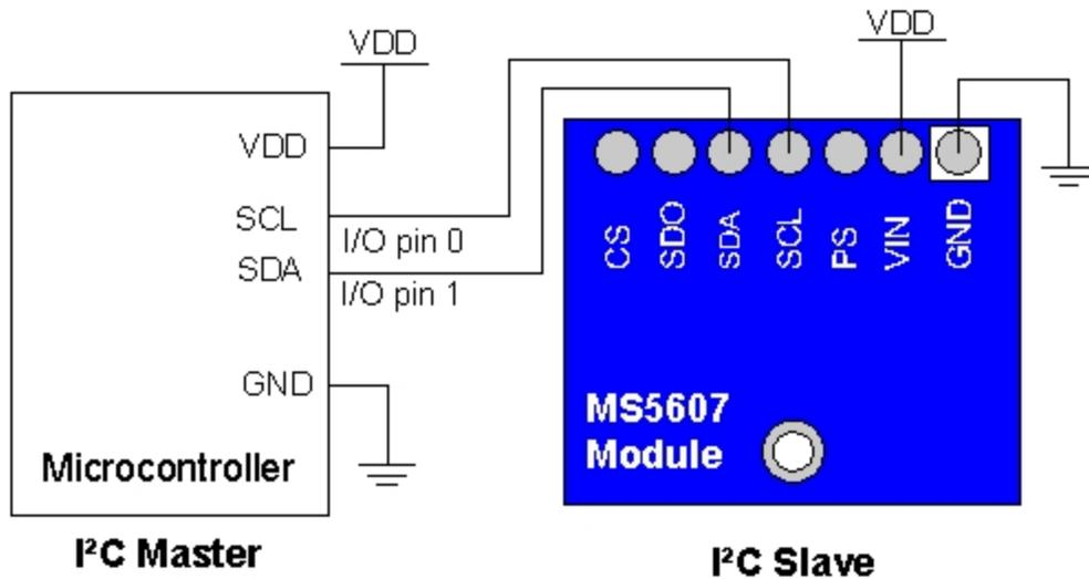
1. With main power off, make the proper connections between the module and a microcontroller as shown below. The voltage connected to the VIN pin should be the same as the voltage powering the microcontroller communicating with the device.
