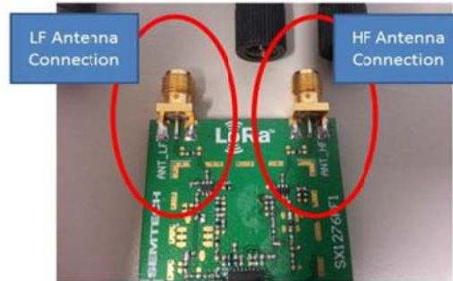
Figure 6: LF and HF Antenna Connection
