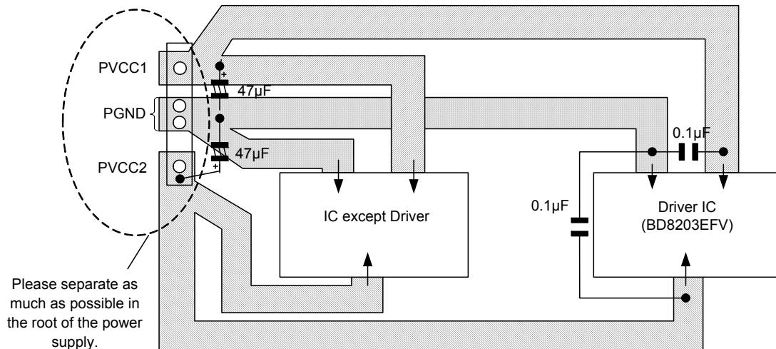
③There is a method of inserting LC filter in the power supply line or GNT line, when not improved by ①②.
