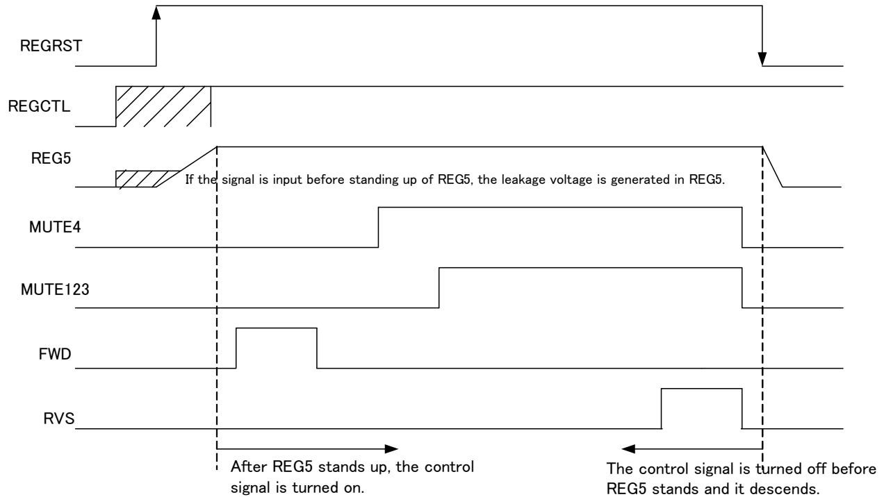
Terminal  $\times$  where the destination of hanging the diode on the power supply side is REG5 must defend the above-mentioned sequence so as not to impress the voltage more than the voltage of REG5 terminal.
