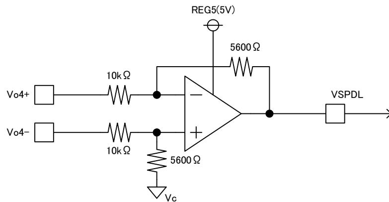
The voltage difference of Vo4+, Vo4- of the BTL driver for SPDL is detected and it outputs to VSPDL terminal.
