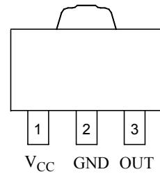
Figure 2. Pin Configuration of AZ70XX (Top View)
