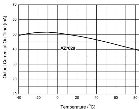
Figure 9. Output Current at On Time vs. Temperature
