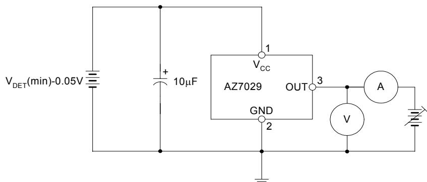
Figure 6. Test Circuit 3
