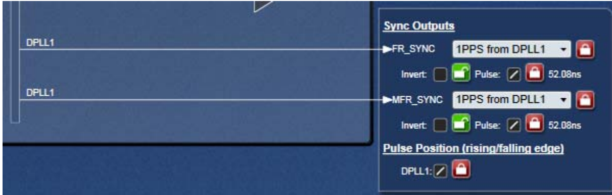
Figure 17. Configure MRSYNC and MRFRSYNC
