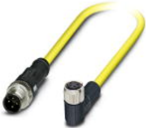
Sensor/Actuator cable, 4-position, PVC, Yellow RAL 1021, Plug straight M12-SPEEDCON, A-coded, on Socket angled M8, Cable length: 0.5 m
