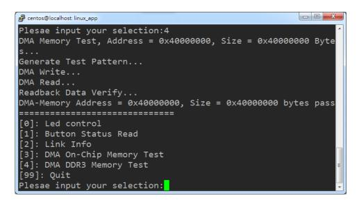
Figure 8-14 DDR3 Memory DMA Test Result
