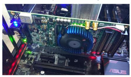
Figure 7-8 FPGA board installation on PC
