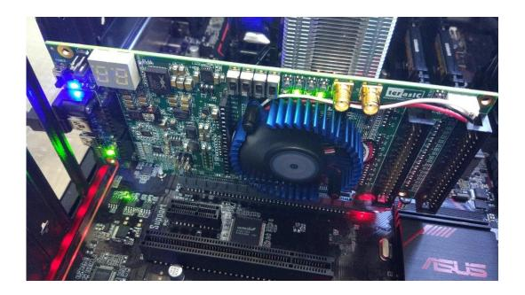
Figure 8-4 FPGA board installation on PC
