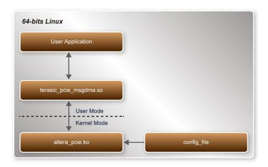
Figure 8-2 PCle Software Stack
