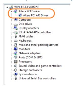
Figure 7-7 Altera PCI API Driver in Device Manager
