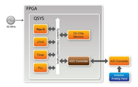
Figure 5-17 ADC System Block Diagram
