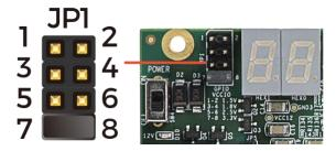
Figure 3-22 Short pin 7 and pin 8 of JP1
