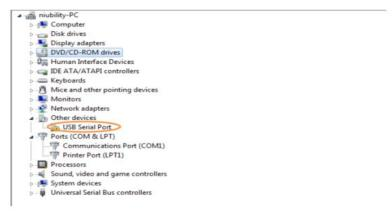
Figure 5-9 Unrecognized USB Serial Port on PC
