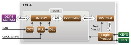
Figure 5-5 Block Diagram of DDR3 Demostration
