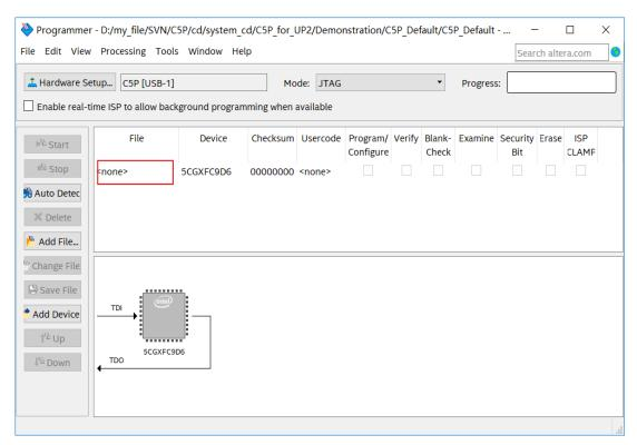
Figure 6-6 Quartus Prime Programmer detecte FPGA device
