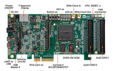
Figure 2-1 C5P development board (top view)
