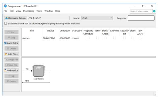
Figure 3-4 FPGA detected in Quartus programmer
