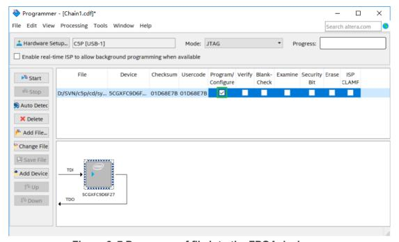
Figure 3-7 Program .sof file into the FPGA device
