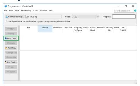
Figure 3-2 Detect FPGA device in JTAG mode
