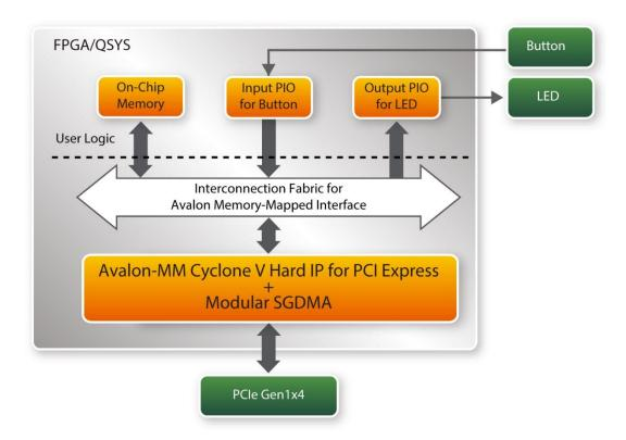
Figure 7-14 Hardware block diagram of the PCle reference design
