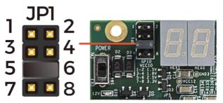
Figure 3-21 Short pin5 and pin 6 of JP1
