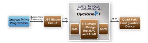
Figure 3-8 Programming a quad serial configuration device with SFL solution
