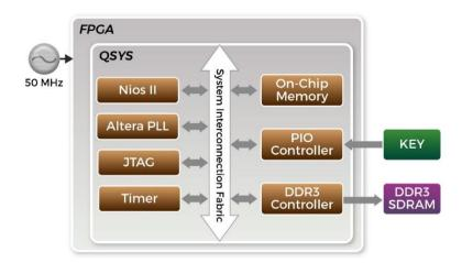
Figure 5-6 Block diagram of the DDR3 Demonstration
