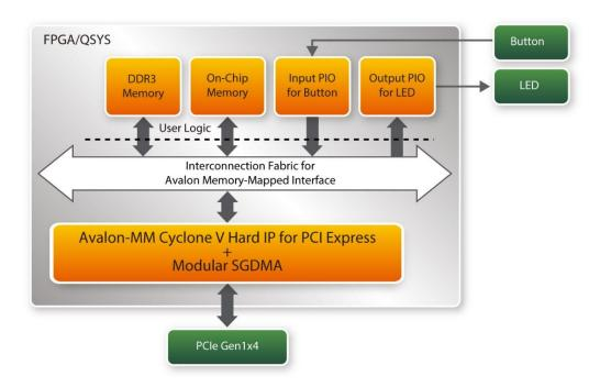
Figure 7-19 Hardware block diagram of the PCle DDR3 reference design
