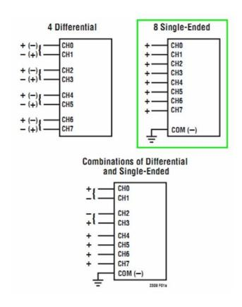
Figure 5-19 Example MUX Configurations
