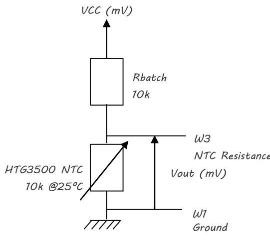
$$V_{OUT}(mV) = \frac{V_{cc}(mV) * NTC_{HTG3500}(\Omega)}{R_{batch}(\Omega) + NTC_{HTG3500}(\Omega)}$$
