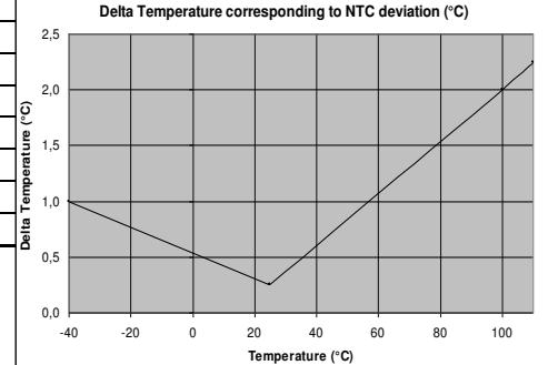
0.1°C tolerance on Resistance Measurement
