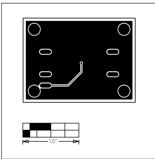
Figure 4. MAX9928 EV Kit PCB Layout—Solder Side
