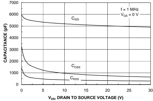
**Figure 8. Capacitance Characteristics**
