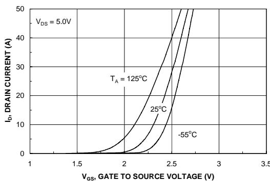
**Figure 5.** Transfer Characteristics
