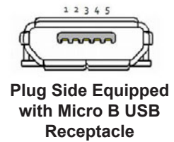
Face View Of Plug As Viewed From Engaging End.
