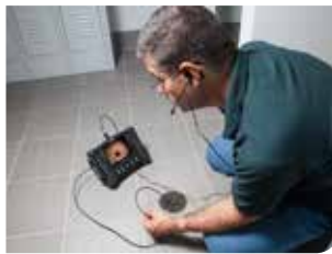
Record video with audio during pipe inspections
