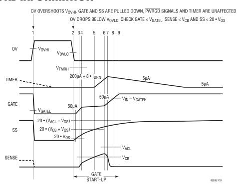
Figure 10. Overvoltage Timing (All Waveforms Are Referenced to V<sub>EE</sub>)
