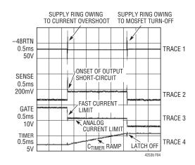
Figure 4. Output Short-Circuit Behavior of LTC4253B
