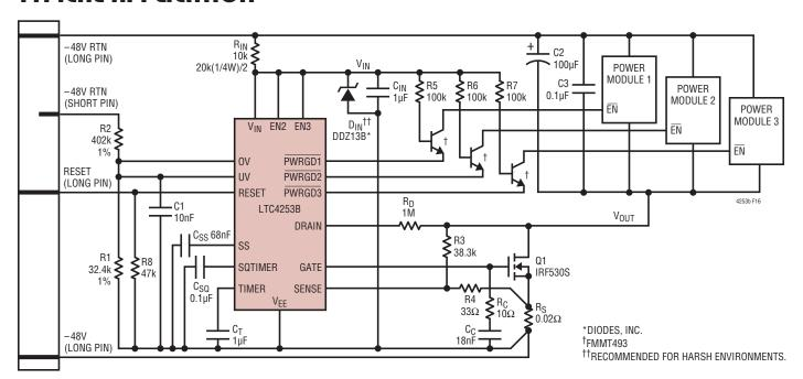
Figure 16. -48V/2.5A Application with Foldback Current Limiting and Transistor Enabled Sequencing without Feedback
