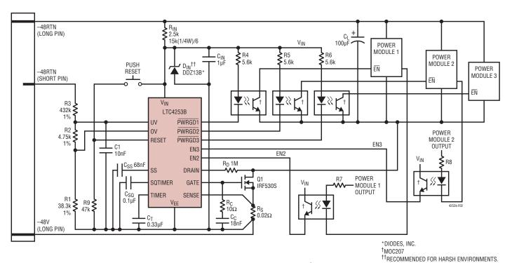
Figure 2. -48V/2.5A Application with a Wider Operating Range
