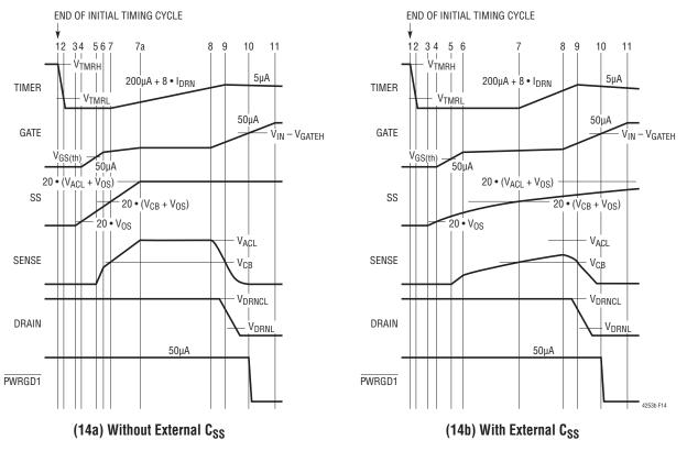
Figure 14. Soft-Start Timing (All Waveforms Are Referenced to V<sub>EE</sub>)
