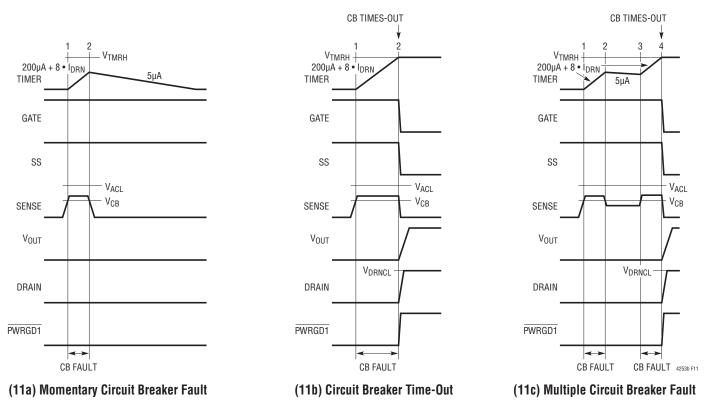
Figure 11. Circuit Breaker Timing Behavior (All Waveforms Are Referenced to VEE)
