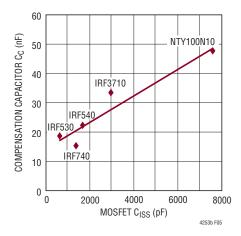
Figure 5. Recommended Compensation Capacitor  $\text{C}_{\text{C}}$  vs MOSFET  $\text{C}_{\text{ISS}}$  for the LTC4253B
