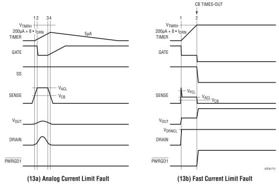
Figure 13. Current Limit Behavior (All Waveforms Are Referenced to V<sub>EE</sub>)
