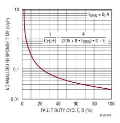
Figure 3. Circuit Breaker Response Time
