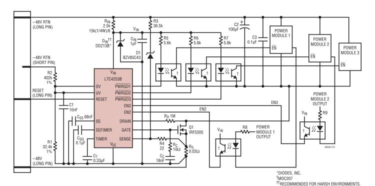
Figure 15. Power Limit Circuit Breaker Application
