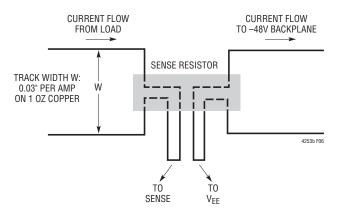
Figure 6. Making PCB Connections to the Sense Resistor
