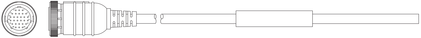
Y Series Motor Static Feedback Cable and Y Series Continuous Flexing Cable P27603-MXX P28122-MXX
