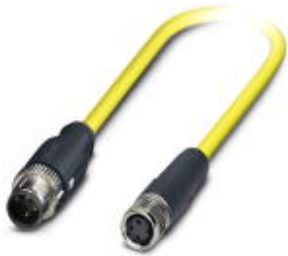
Sensor/Actuator cable, 3-position, PVC, yellow, shielded, Plug straight M12-SPEEDCON, A-coded, on Socket straight M8, Cable length: 0.5 m
