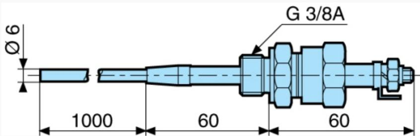
Electrode holder with a single probe supplied in a standard length of 1000mm. (304 stainless steel). Mounting with external 3/8" BSP thread and hexagonal head. Use 24 mm. spanner for hexagon. Suitable for use on boilers, autoclaves and under high temperature conditions up to 200 °C and high pressure conditions up to 25 kg/cm<sup>2</sup>
