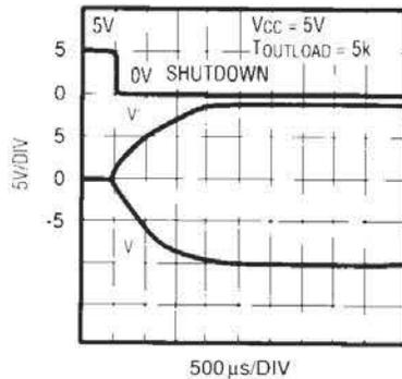
**RTRI DELAY TIME TO RECEIVER OUTPUT ACTIVE**
