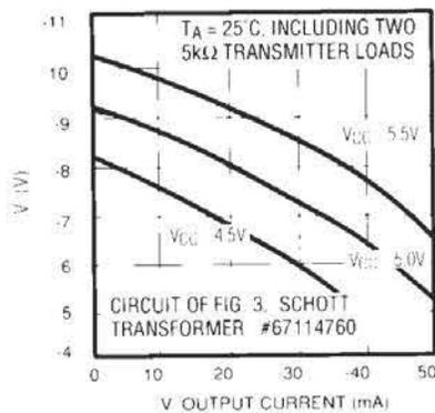
**MAX251  $V^-$  BYPASS vs. LOAD**
