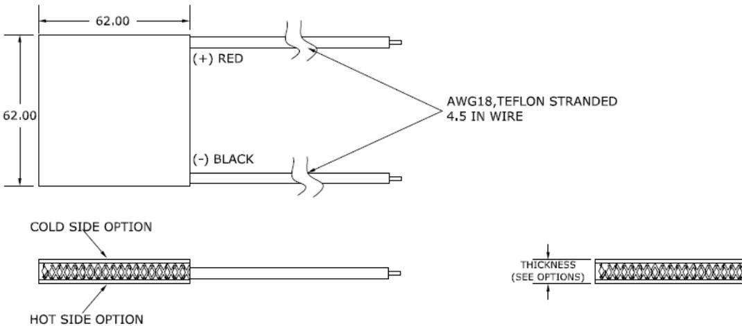
Ceramic Material: Alumina( $\text{Al}_2\text{O}_3$ )
