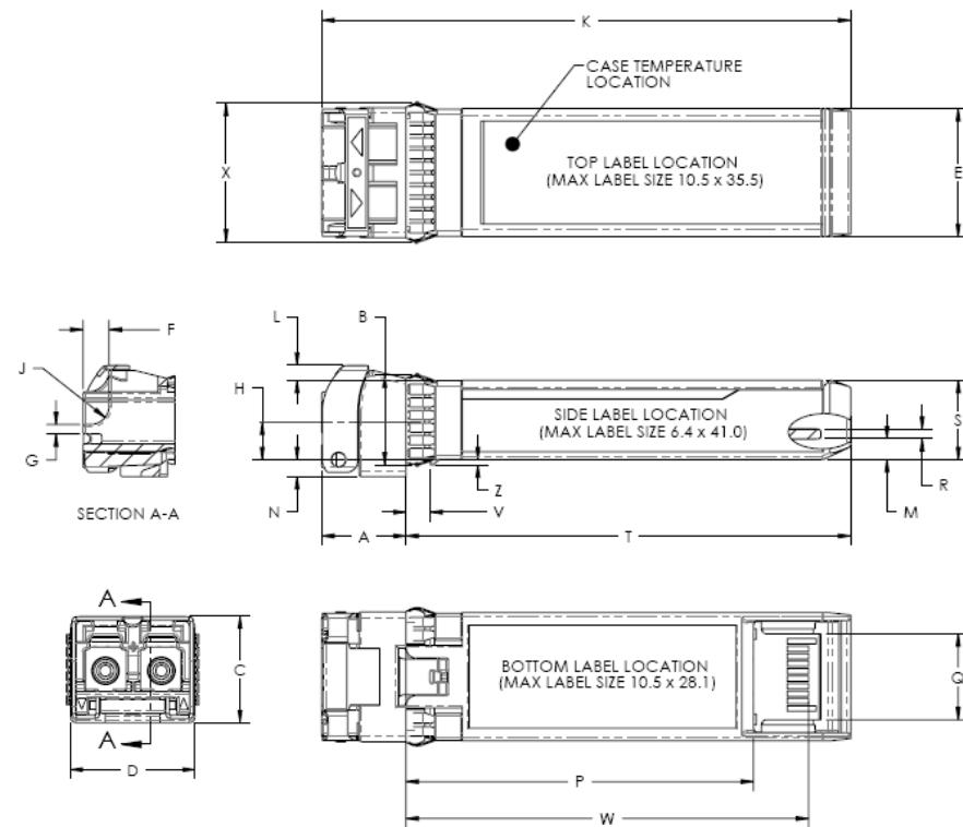
Figure 2. Mechanical Dimensions
