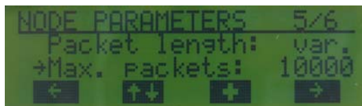
Figure 12. Menu Page: Node Parameters 5/6 (Rx mode)
