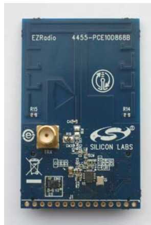
Figure 2. Si4455 RF Pico Board—868 MHz (P/N 4455-PCE10D868B)
