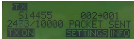
Figure 16. Running PER Test (Tx Mode)
