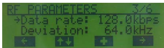
Figure 8. Menu Page: RF Parameters 3/6 (Modulation is 2GFSK)
