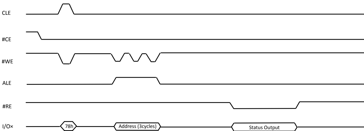
Figure 9-11 Read Status Enhanced (78h) Operation
