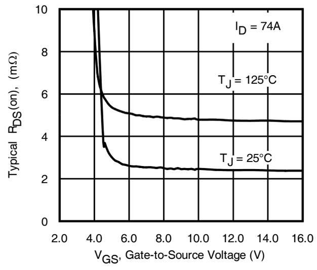
**Fig. 3** Typical On-Resistance vs. Gate Voltage
