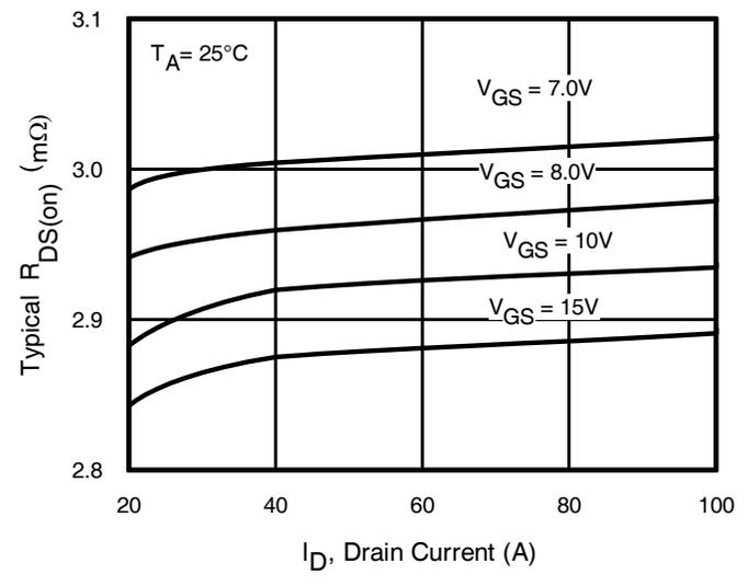
**Fig. 4** Typical On-Resistance vs. Drain Current
