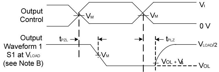
Voltage Waveform Enable and Disable Times
