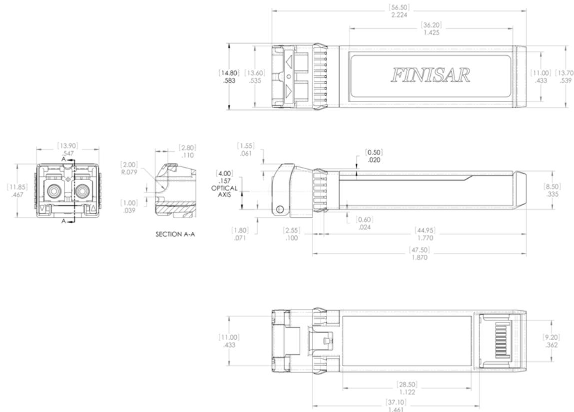
**Figure 2. FTLX8573D3BTL Mechanical Dimensions.**
