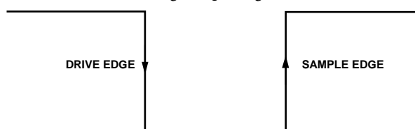
Figure 41. SPI Mode 3 SCLK Edges
