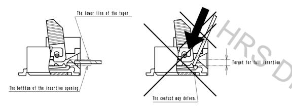
Do not apply force to the actuator during FPC full insertion procedure. FPC insertion could become stiff and/or difficult for wiping.
