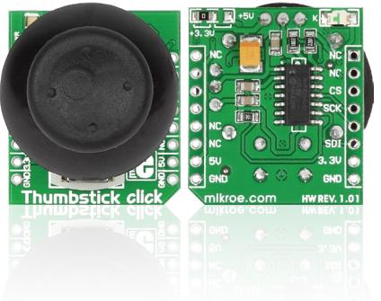
Thumbstick click™ is a simple solution for adding an analog thumb joystick to your design. Along with the dual axis joystick unit, the board also carries an **MCP3204** 12-bit A/D converter. Thumbstick click™ communicates with the target board microcontroller through **mikroBUS™** SPI (CS, SCK, MISO and MOSI) lines. The board is designed to use either a 3.3V or a 5V power supply.
