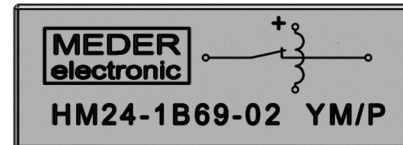
Marking according to EN60062/factory code gem. EN60062/Fertigungsstätte
