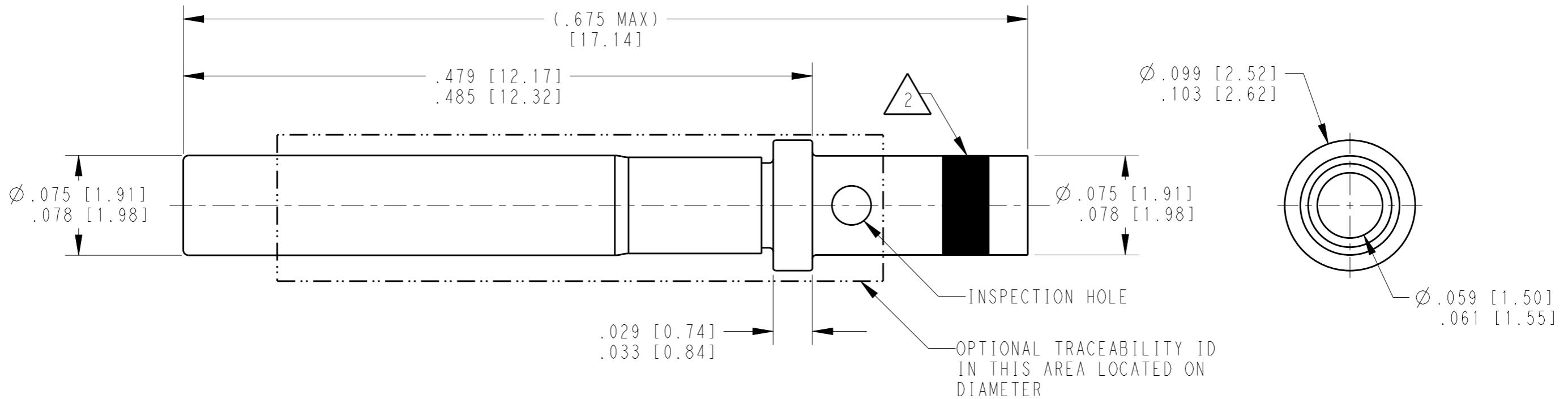
3. WIRE RANGE : 18 AWG TO 16 AWG [0.75 - 1.0 mm<sup>2</sup>]
