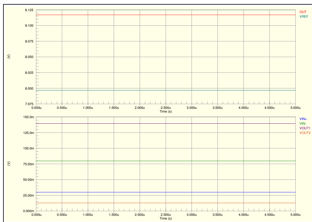
FIGURE 2-18: Simulation of the DC Response.
