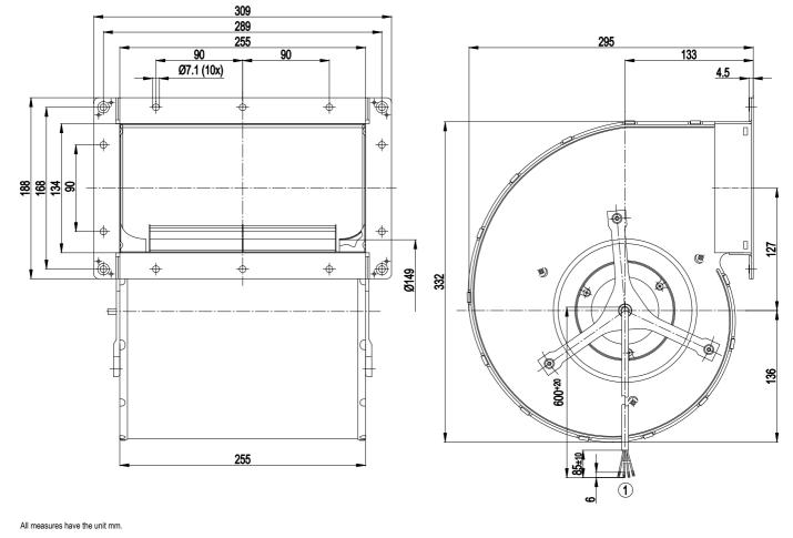
Connection line PVC 4G 0.5 mm<sup>2</sup>, 4x brass lead tips crimped
