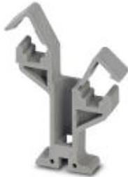
Double support, insulating material, optionally for use with 3 mm x 10 mm or 6 mm x 6 mm busbar, height: 48 mm
