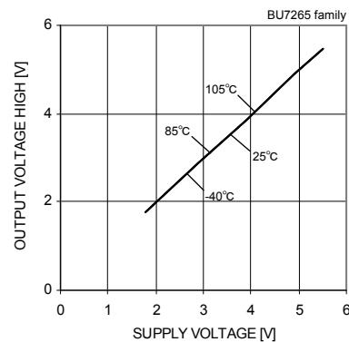
Fig.5 Output Voltage High – Supply Voltage ( $RL=10[k\Omega]$ )
