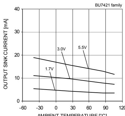
Fig.81 Output Sink Current
