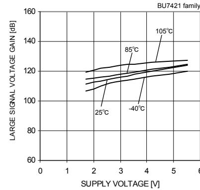
Fig.85 Large Signal Voltage Gain
