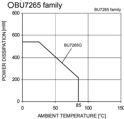
Fig.1 Derating curve
