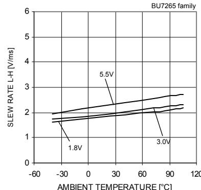
Fig.21 Slew Rate L-H
