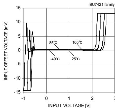
Fig.84 Input Offset Voltage
