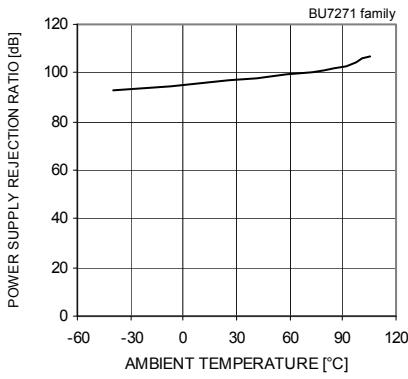
Fig.43 Power Supply Rejection Ratio
