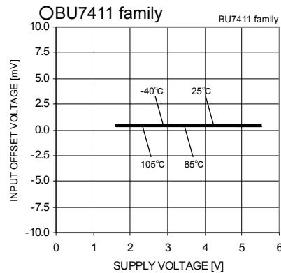
Fig.59 Input Offset Voltage
