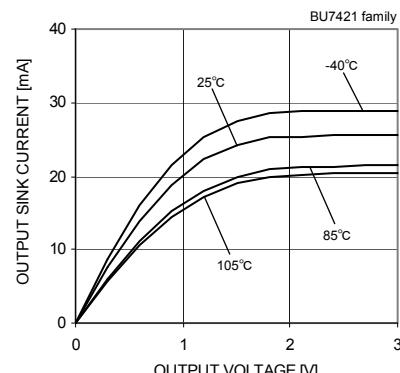
Fig.80 Output Sink Current
