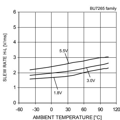
Fig.22 Slew Rate H-L
