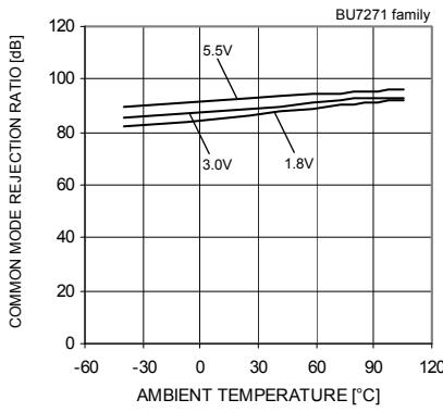
Fig.42 Common Mode Rejection Ratio
