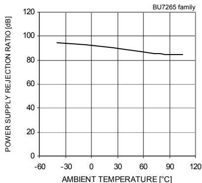
Fig.20 Power Supply Rejection Ratio
