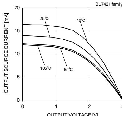
Fig.78 Output Source Current
