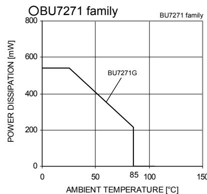
Fig.24 Derating curve
