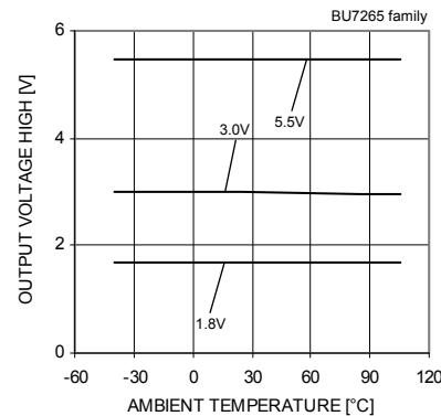
Fig.6 Output Voltage High – Ambient Temperature ( $RL=10[k\Omega]$ )
