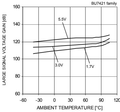
Fig.86 Large Signal Voltage Gain
