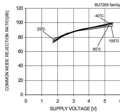
Fig.18 Common Mode Rejection Ratio
