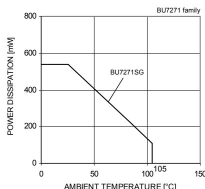
Fig.25 Derating curve
