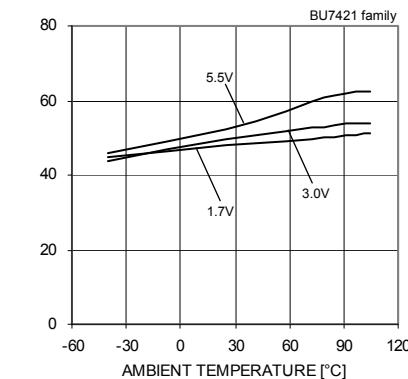
Fig.90 Slew Rate L-H
