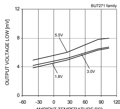
Fig.31 Output Voltage Low – Ambient Temperature (RL=10[kΩ])
