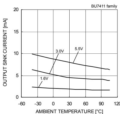
Fig.58 Output Sink Current
