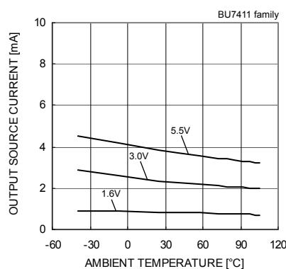
Fig.56 Output Source Current
