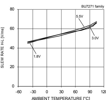
Fig.45 Slew Rate H-L
