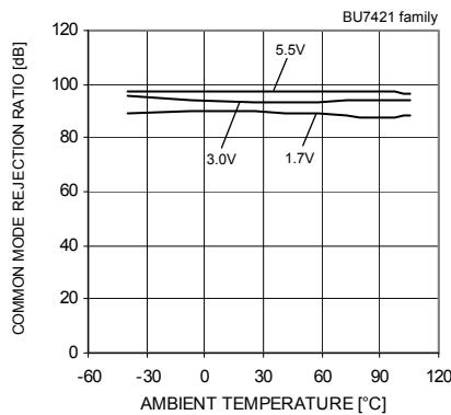
Fig.88 Common Mode Rejection Ratio
