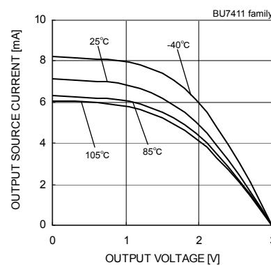
Fig.55 Output Source Current
