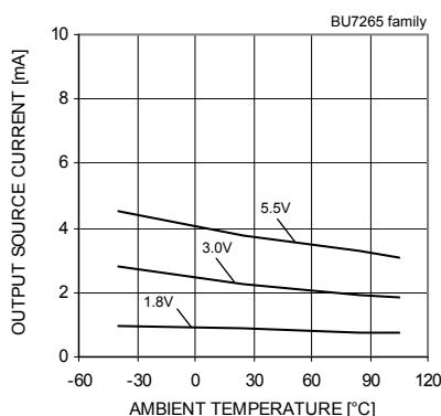
Fig.10 Output Source Current – Ambient Temperature ( $VOUT=VDD-0.4[V]$ )
