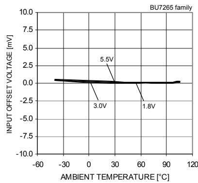
Fig.14 Input Offset Voltage –
