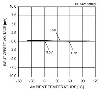
Fig.83 Input Offset Voltage
