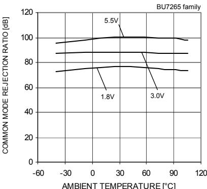
Fig.19 Common Mode Rejection Ratio
