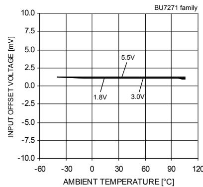
Fig.37 Input Offset Voltage
