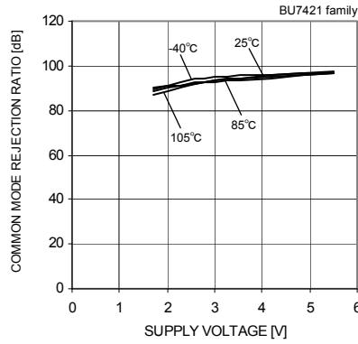
Fig.87 Common Mode Rejection Ratio
