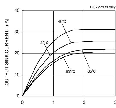
Fig.34 Output Sink Current
