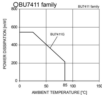
Fig.47 Derating curve
