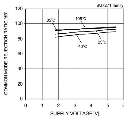
Fig.41 Common Mode Rejection Ratio
