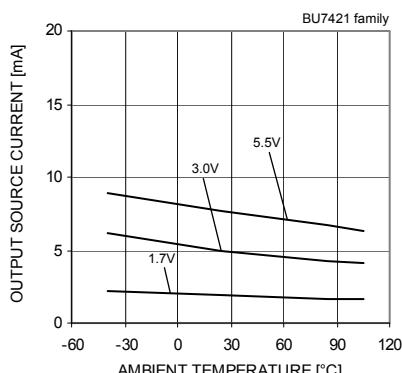
Fig.79 Output Source Current
