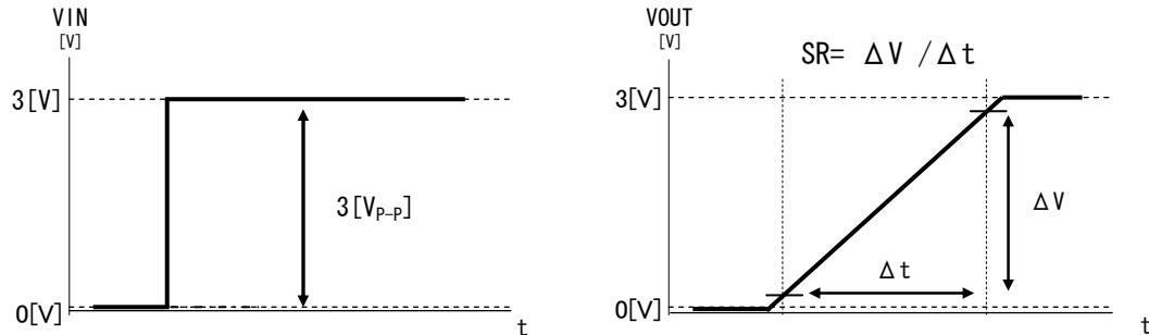
Fig.96 Slew rate input output wave
