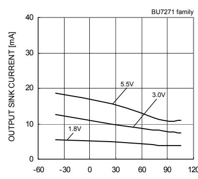
Fig.35 Output Sink Current
