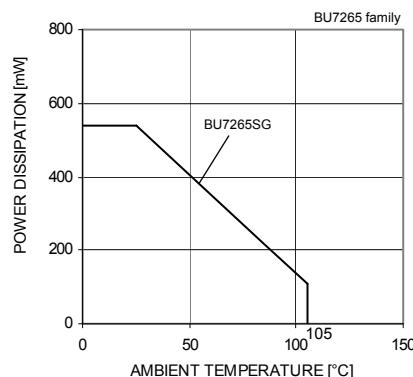
Fig.2 Derating curve
