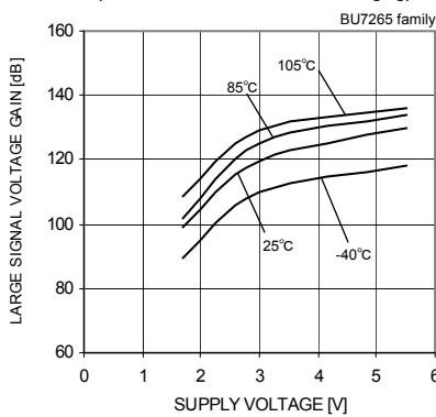
Fig.16 Large Signal Voltage Gain
