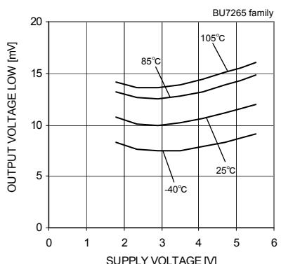
Fig.7 Output Voltage Low – Supply Voltage ( $RL=10[k\Omega]$ )
