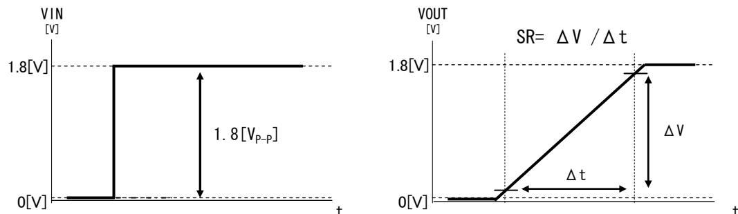
Fig.97 Slew rate input output wave
