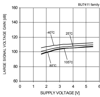
Fig.62 Large Signal Voltage Gain
