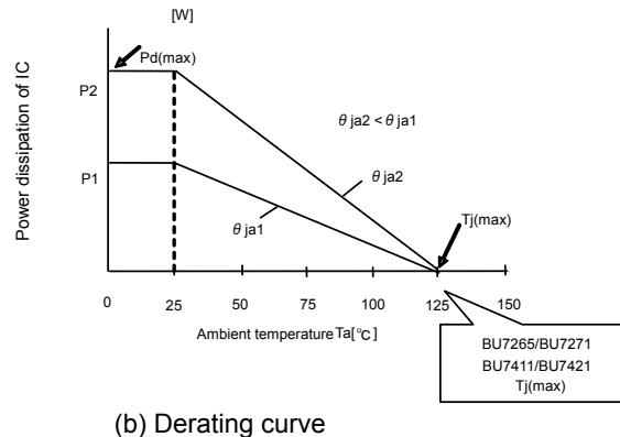
Fig.98 Thermal resistance and derating
