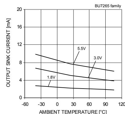
Fig.12 Output Sink Current – Ambient Temperature ( $VOUT=VSS+0.4[V]$ )
