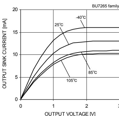
Fig.11 Output Sink Current – Output Voltage ( $VDD=3[V]$ )
