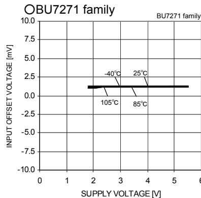
Fig.36 Input Offset Voltage
