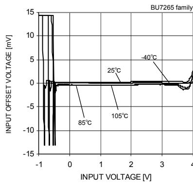
Fig.15 Input Offset Voltage
