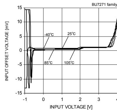
Fig.38 Input Offset Voltage – Input
