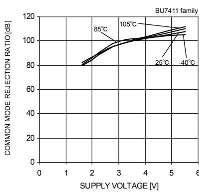
Fig.64 Common Mode Rejection Ratio
