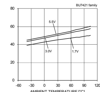
Fig.91 Slew Rate H-L
