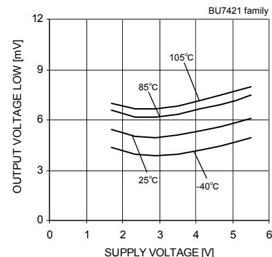
Fig.76 Output Voltage Low – Supply Voltage (RL=10[kΩ])
