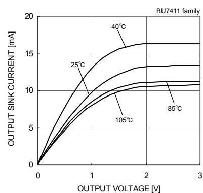
Fig.57 Output Sink Current
