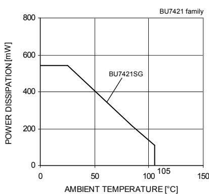
Fig.71 Derating curve
