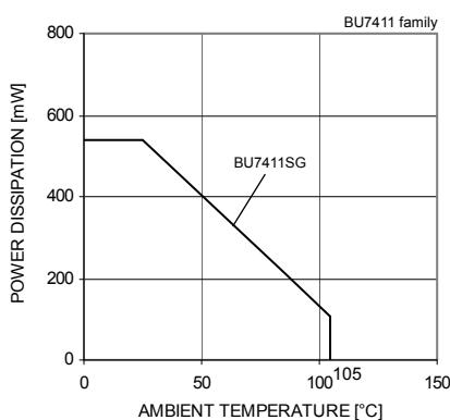
Fig.48 Derating curve
