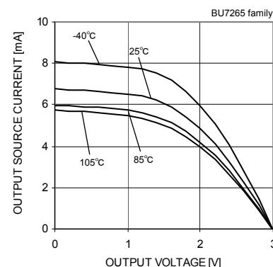
Fig.9 Output Source Current – Output Voltage ( $VDD=3.0[V]$ )
