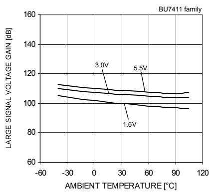
Fig.63 Large Signal Voltage Gain
