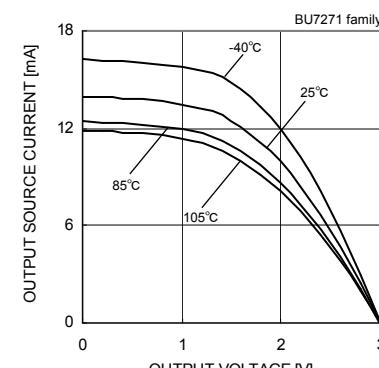
Fig.32 Output Source Current –
