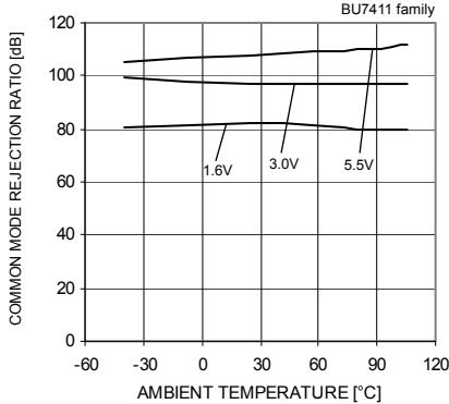
Fig.65 Common Mode Rejection Ratio
