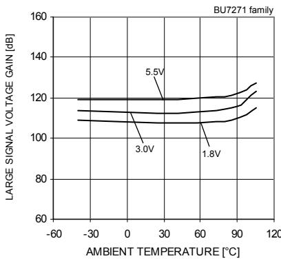
Fig.40 Large Signal Voltage Gain
