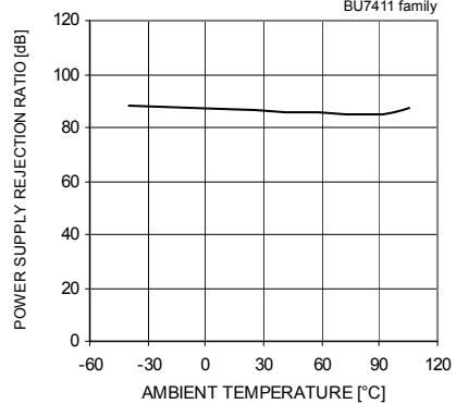
Fig.66 Power Supply Rejection Ratio
