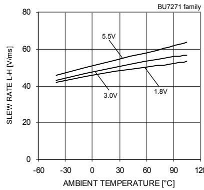
Fig.44 Slew Rate L-H
