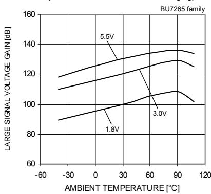
Fig.17 Large Signal Voltage Gain
