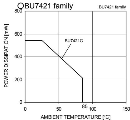
Fig.70 Derating curve
