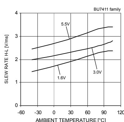
Fig.68 Slew Rate H-L
