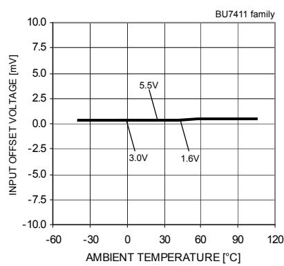
Fig.60 Input Offset Voltage
