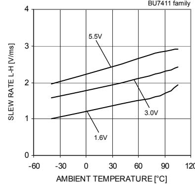
Fig.67 Slew Rate L-H
