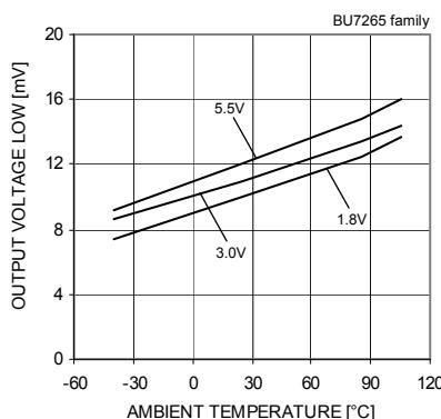
Fig.8 Output Voltage Low – Ambient Temperature ( $RL=10[k\Omega]$ )
