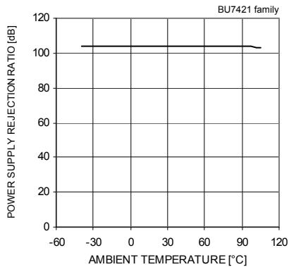
Fig.89 Power Supply Rejection Ratio
