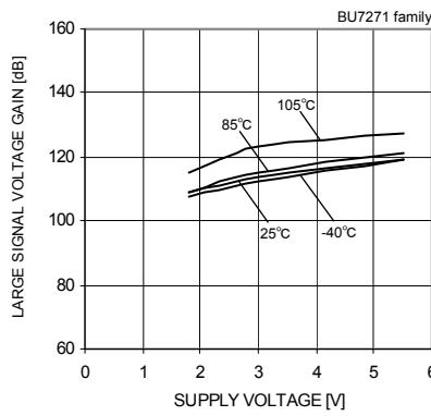
Fig.39 Large Signal Voltage Gain
