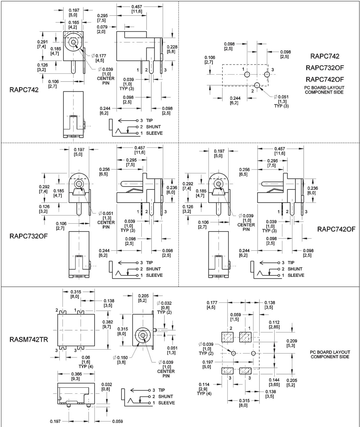
DIMENSIONS ARE FOR REFERENCE ONLY  $\frac{\text{Inch}}{(\text{mm})}$
