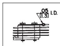
**Bussing type terminals which allow you to buss jacks quickly and easily are available on special order.**
