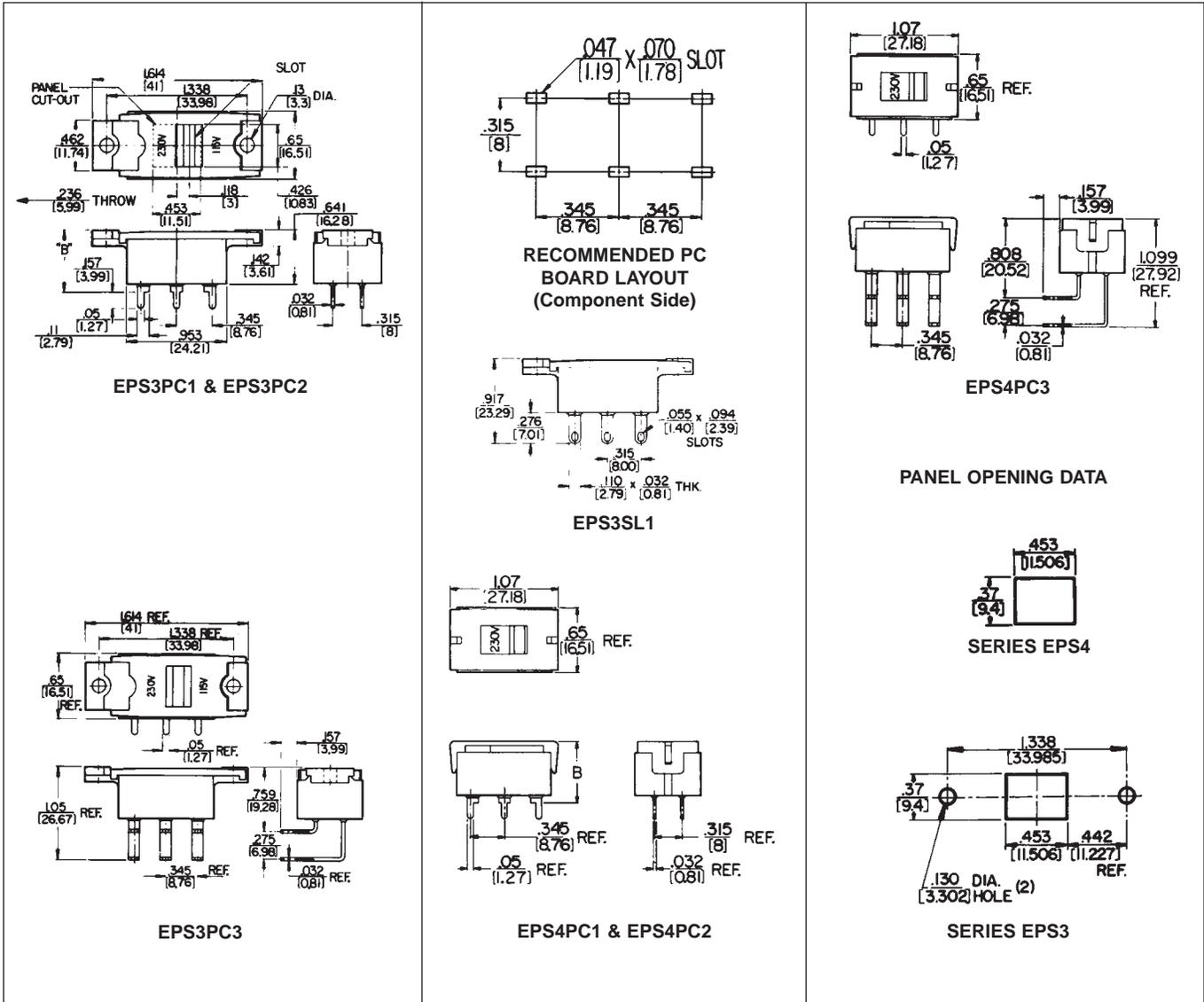
DIMENSIONS ARE FOR REFERENCE ONLY  $\frac{\text{Inch}}{\text{(mm)}}$
