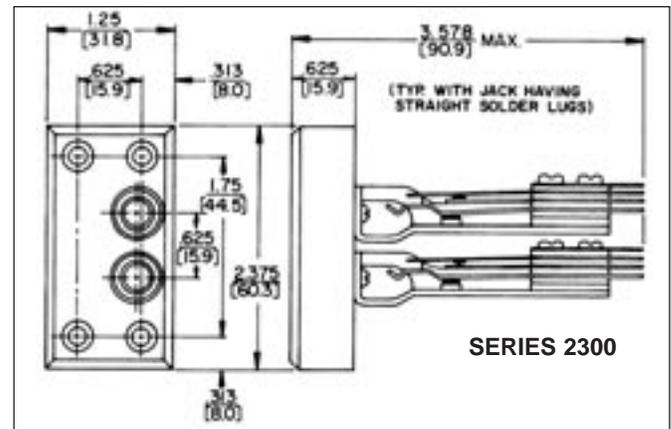
DIMENSIONS ARE FOR REFERENCE ONLY  $\frac{\text{Inch}}{\text{(mm)}}$
