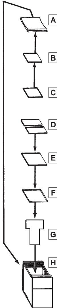
**SERIES 401 DISPLAY SCREENS** – Display screens with contoured face give a better operation “feel”. Rectangular shape provides greater area for engraving legends and symbols. Entire screen is illuminated by single or twin lamp indication. Various brightness and color combinations are possible by use of legend filter and split face inserts.
