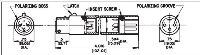
Male-female connector conversion has male Q-G® insert at one end and corresponding female Q-G® insert at the other. Designed to accept internally connected transformer, attenuator, or other circuitry inline with microphone input. Includes 1.50" (38.1 mm) long x .594" (15.08 mm) diameter of usable internal volume.
