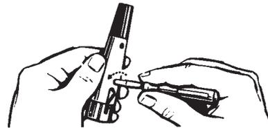
Insert screw engages as any conventional screw, except it is lefthand threaded. To disassemble the connector, turn screw counterclockwise down into insert (see illustration).
