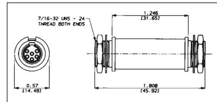
3-6 pin male-to-male adapter is designed for through-bulkhead or cable expansion usage. Adapter is prewired pin 1 to pin 1, pin 2 to pin 2, etc. Mounting nuts are supplied for each threaded end. Panel hole diameter required is .45"; maximum panel thickness is .25" (6.35 mm).
