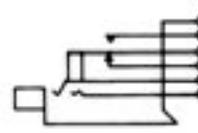
Double open circuit. Isolated switching—"break" before "make" circuit.
