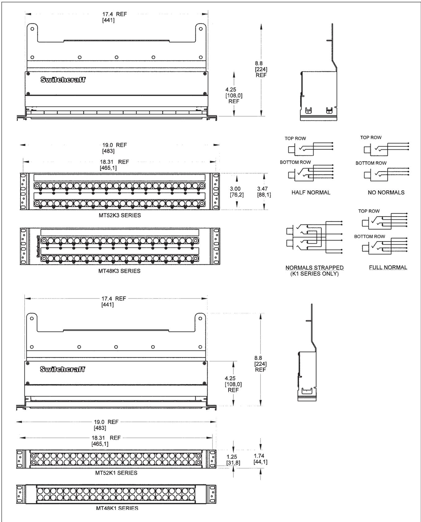
DIMENSIONS ARE FOR REFERENCE ONLY  $\frac{\text{Inch}}{\text{(mm)}}$
