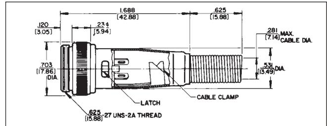
Non-reflective metal shell; 2 through 5 pins (male) or 2 through 5 contacts (female). Also 2-, 3- and 4-contact inserts with two shunted (N.C.) contacts. Efficient cable clamp and strain relief.
