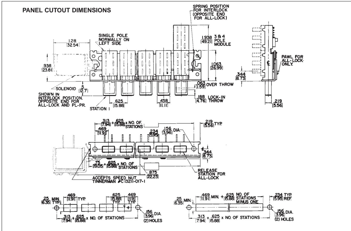
DIMENSIONS ARE FOR REFERENCE ONLY  $\frac{\text{Inch}}{\text{(mm)}}$
