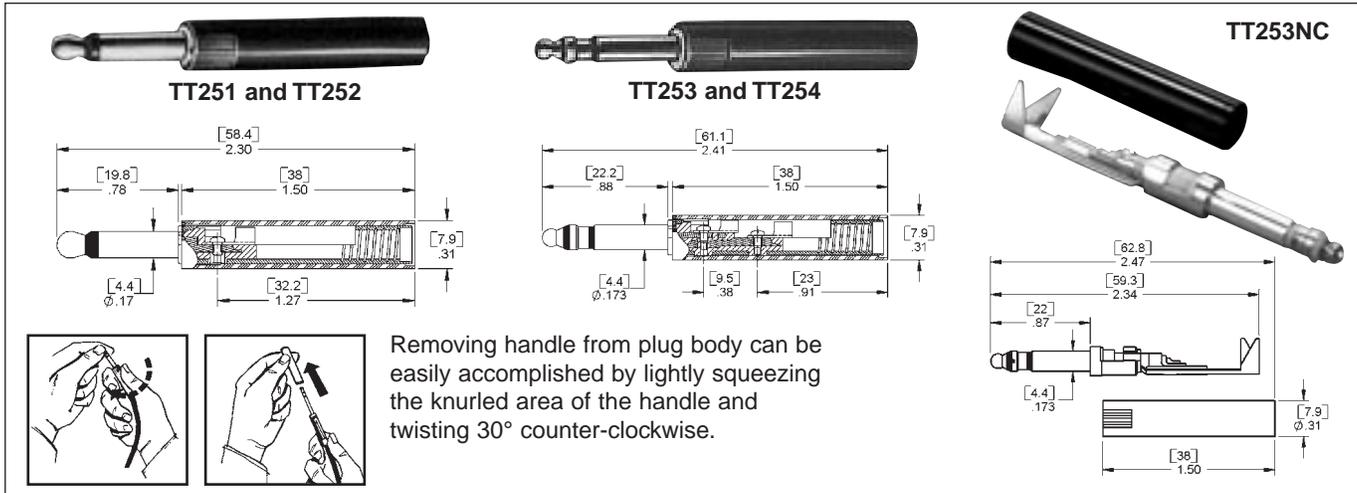
Removing handle from plug body can be easily accomplished by lightly squeezing the knurled area of the handle and twisting 30° counter-clockwise.
