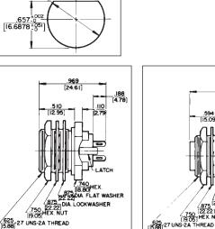
Rear of panel mount; 2 through 5 pins (male) or 2 through 5 contacts (female). Also 2-, 3- and 4-contact inserts with 2 shunted (N.C.) contacts. Mounting locknut (Part Number SL01), lock washer (Part Number SL02), and flat washer (Part Number SL03) supplied.
