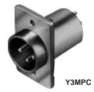
**Series Y(\*)MPC.** Male receptacle for panel or chassis mounting escutcheon. PC terminals and standoffs. Rear of panel mount in .750 inch diameter hole. Maximum panel thickness: 25 inches (6.35 mm); .156 inches (3.96 mm) if YEM escutcheon is used.
