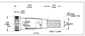
Non-reflective metal shell; coupling ring; 2 through 5 pins (male) or 2 through 5 contacts (female). Also 2-, 3- and 4-contact inserts with two shunted (N.C.) contacts. Efficient cable clamp and strain relief.
