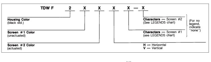
TDW-F "FLIP-FLOP" PUSHBUTTON PART NUMBERING
