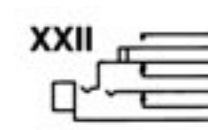
Double closed circuit. Isolated switching "make" circuit on ring spring. (J7-1A).
