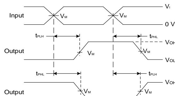
**Voltage Waveform Propagation Delay Times
