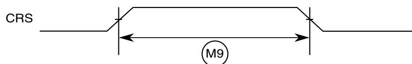
Figure 43. MII async inputs timing diagram
