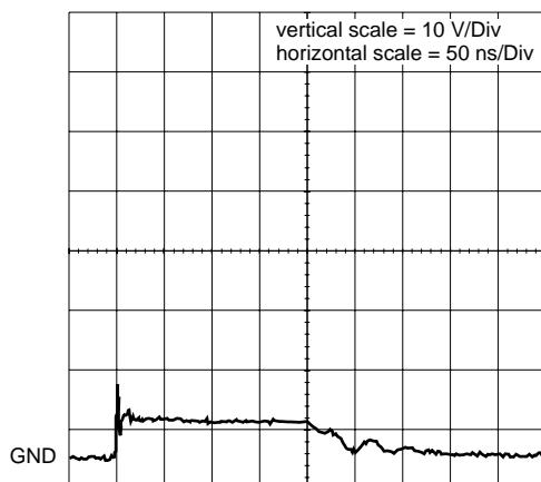
clamped +1 kV ESD voltage waveform
