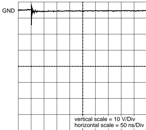
clamped -1 kV ESD voltage waveform
