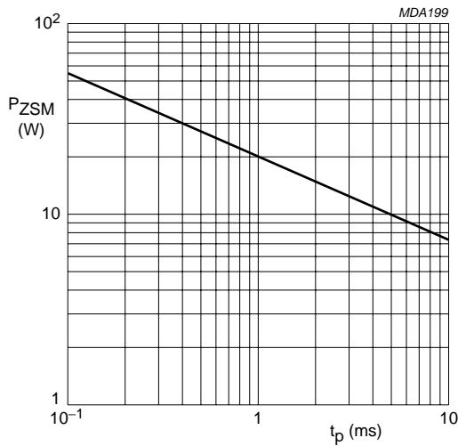
$P_{ZSM} = V_{ZSM} \times I_{ZSM}$ .
