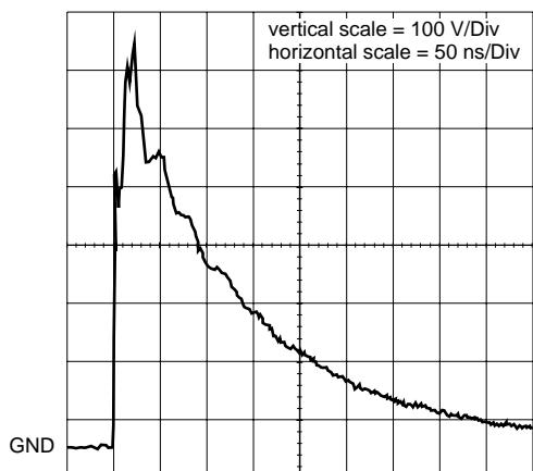
unclamped +1 kV ESD voltage waveform
