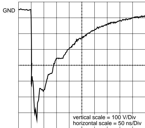
unclamped -1 kV ESD voltage waveform
