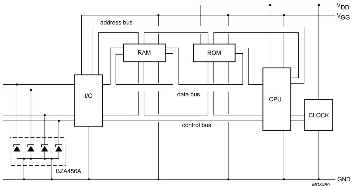
Fig.8 Microprocessor protection.
