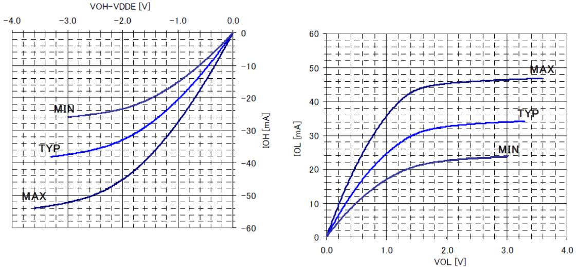
Apply to pins CLKOUT, TXRX0, TXRX1
