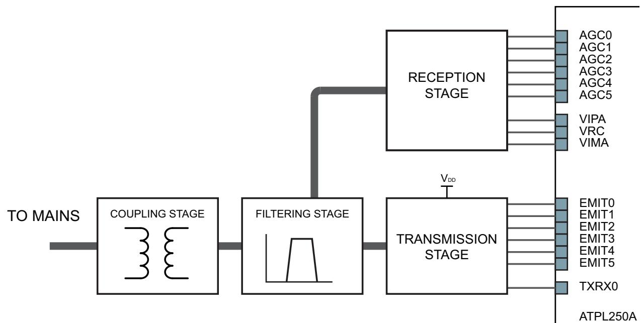
A particular reference design can contain more than one sub-circuit of the same kind (i.e.: two transmission stages).
