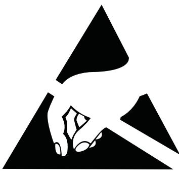
Precautions for handling electrostatic sensitive devices should be taken into account to avoid malfunction. Charged devices and circuit boards can discharge without detection.
