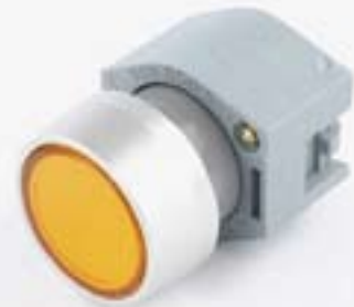
Non-Illuminated raised pushbutton, aluminium bezel, 22.5mm mounting
