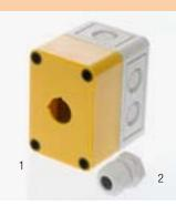
Emergency-stop switch enclosure, with 22.5 mm  $\varnothing$  mounting hole, 94 mm (w) x 65 mm (h) x 81 mm (d), anti twist hole. Cable gland M20, IP66
