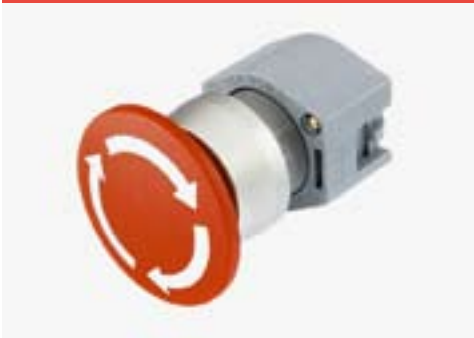
Stop switch, twist release, mushroom head, 40 mm diameter, 22.5 mm mounting
