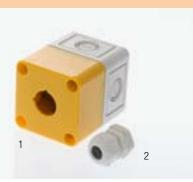
Emergency-stop switch enclosure with 22.5 mm  $\varnothing$  mounting hole, 65 mm (w) x 65 mm (h) x 81 mm (d), anti twist hole. Cable gland M20, IP66
