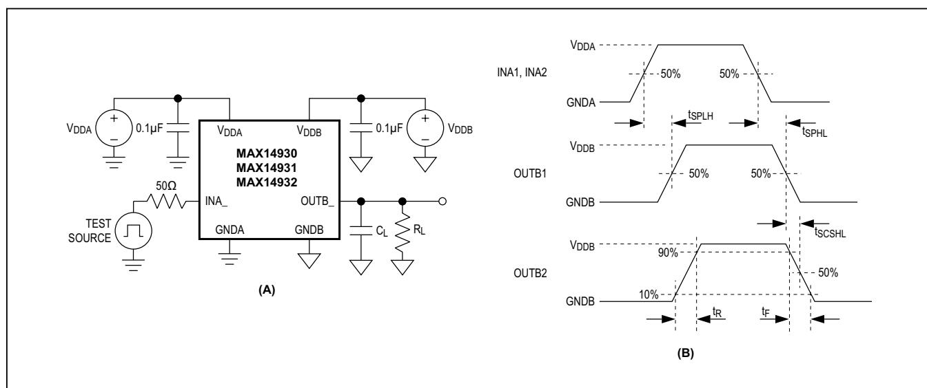
Figure 1. Test Circuit (A) and Timing Diagram (B)
