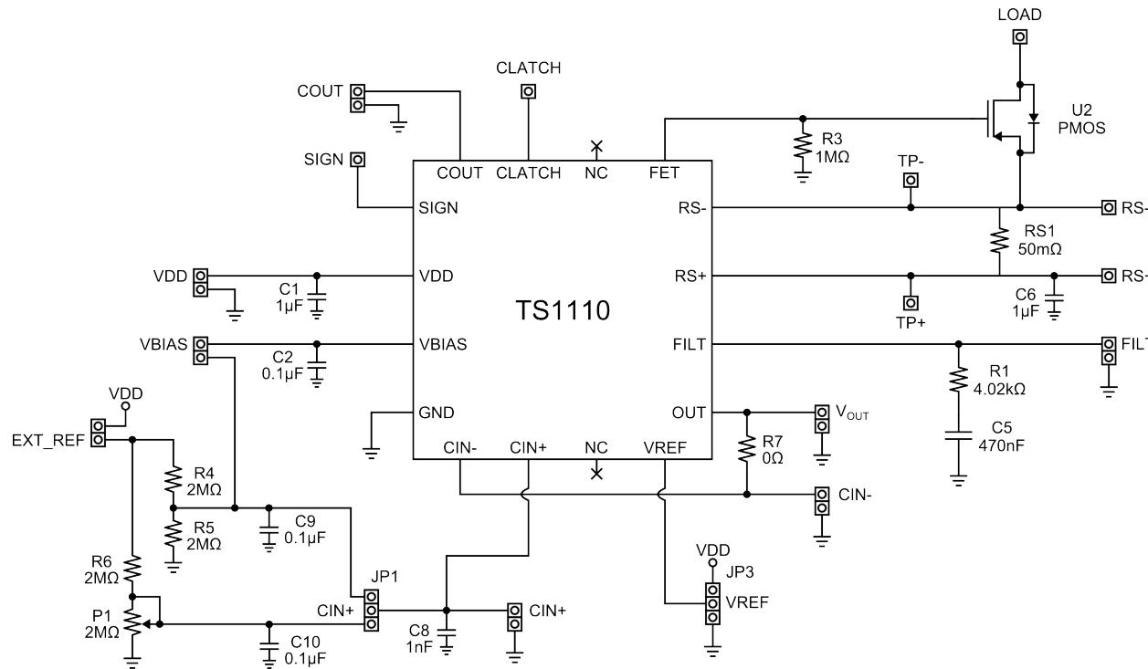
Figure 2.1. TS1110DB Circuit Schematic
