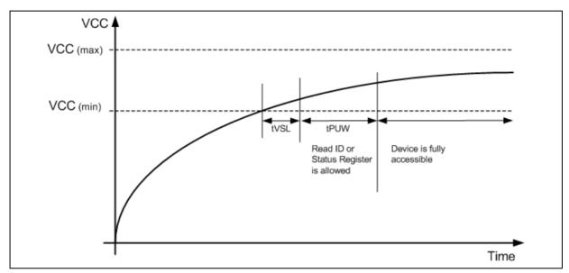
Figure 33a. Power-up Timing and Voltage Levels
