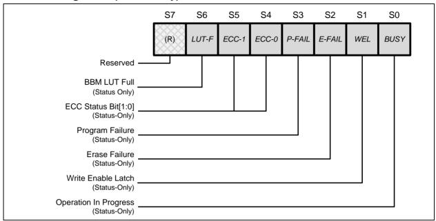
Figure 4c. Status Register-3 (Address Cxh)
