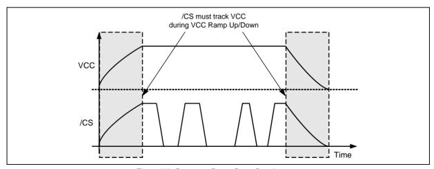
Figure 33b. Power-up, Power-Down Requirement
