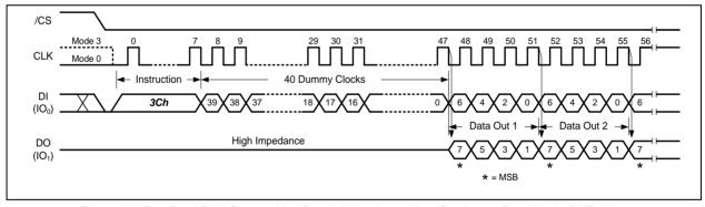
Figure 23b. Fast Read Dual Output with 4-Byte Address Instruction (Continuous Read Mode, BUF=0)
