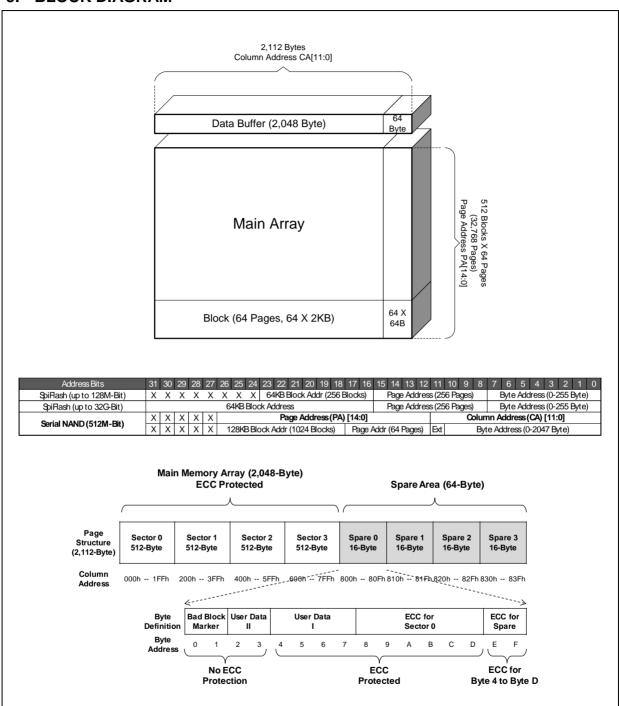
Figure 2. W25N512GW Flash Memory Architecture and Addressing
