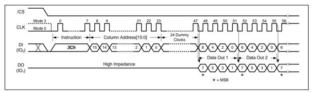
Figure 23a. Fast Read Dual Output with 4-Byte Address Instruction (Buffer Read Mode, BUF=1)
