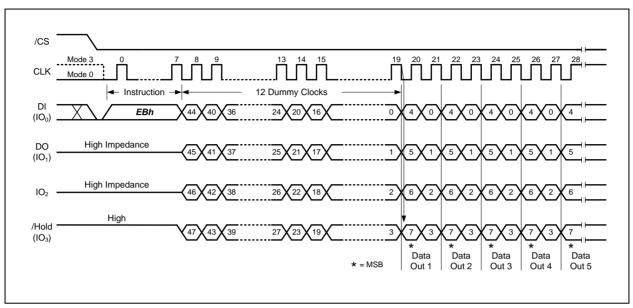
Figure 28b. Fast Read Quad I/O Instruction (Continuous Read Mode, BUF=0)
