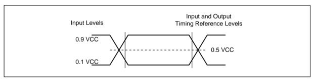
Figure 34. AC Measurement I/O Waveform
