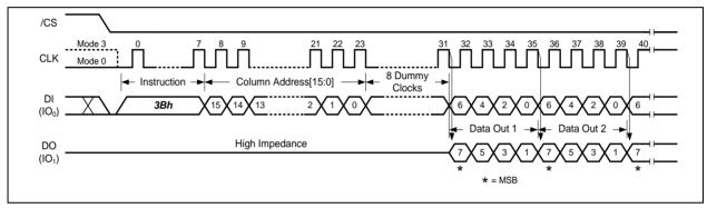
Figure 22a. Fast Read Dual Output Instruction (Buffer Read Mode, BUF=1)
